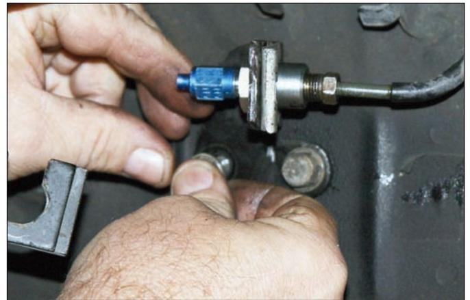
**Sequence 12:** Reinstall the modified bracket in the original position using saved original bolts on the wheel well. Slide the new fitting into the bracket and secure in place with the retaining clip.
