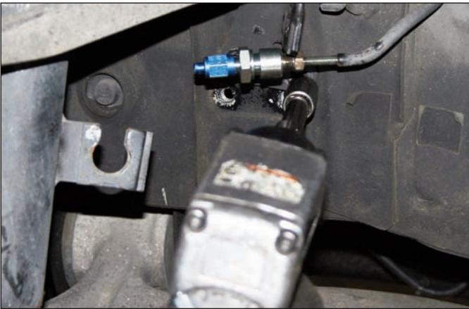
**Sequence 8:** Remove the two bolts (save) that attach the hose line bracket to the inner wheel well adjacent to the hard line where the line fitting was installed earlier.
