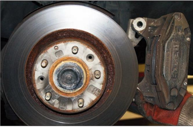
**Sequence 7:** Finish removing the caliper mounting bolts and lift off the caliper. Save bolts for reinstallation. Remember there is still some fluid in the rubber hose attached to the caliper.
