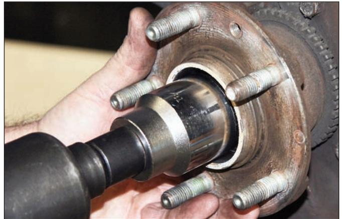
**Sequence 17:** Remove the spindle nut from inside the hub assembly using the corresponding socket size.
