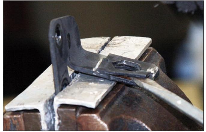
**Sequence 10:** After the welds have been cut, pry off the top plate from the base using a screw driver or chisel.
