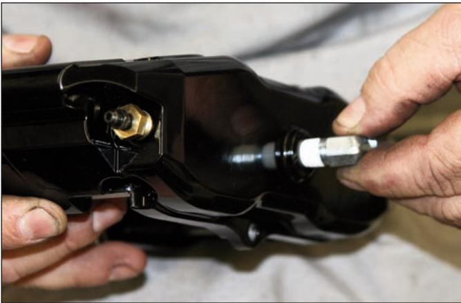
**Sequence 31:** Remove the protective sticker from the caliper fluid inlet. Coat the inlet fitting with PTFE thread tape and screw into the caliper with the 90° angle perpendicular to the length of the caliper.
