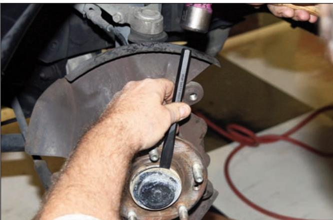
**Sequence 15:** Carefully pry off the dust cap from the face of the hub using a chisel or screw driver and a hammer.
