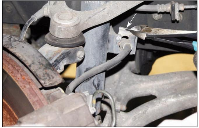
**Sequence 4:** On the backside of the OEM brake hose retaining bracket, remove the clip holding the hose fitting (arrow). Lift the hose up from the bottom portion of the bracket assembly.
