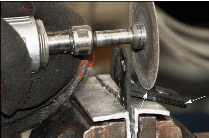
**Sequence 9:** Secure the hose clamp in a vise and grind off the welds on both ends (arrows) that secure the top plate to the base of the bracket. This needs to be done to facilitate the installation of the Wilwood flexline.
