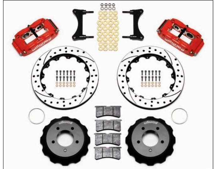
Wilwood part number 140-11963 comes complete with Superlite 6R calipers, caliper mounting brackets, GT rotors, aluminum hats, BP-10 brake pads and all necessary hardware for an easy bolt-on installation.
