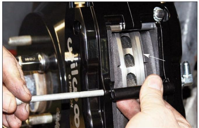
**Sequence 35:** Check that the top of the brake pad is flush with the outside diameter of the rotor (arrow). If not, adjust by adding or subtracting shim between the bracket and the caliper.
