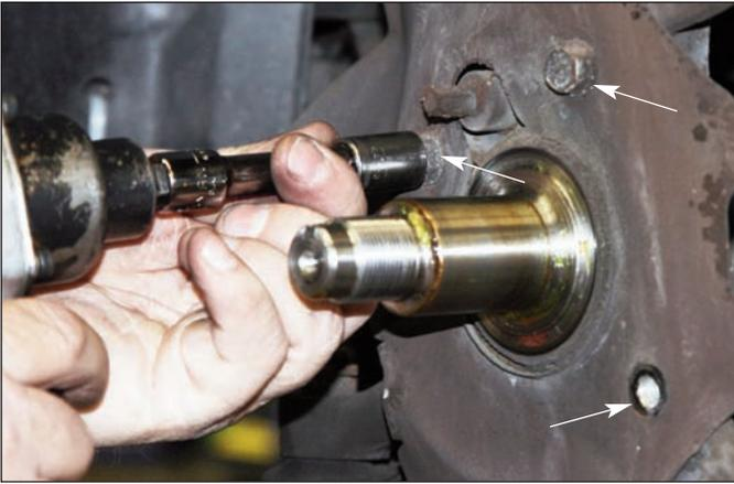
**Sequence 19:** Remove the three bolts (arrows) that hold the dust shield in place. Remove the dust shield and discard, it will not be utilized in the installation of the Wilwood brake kit.
