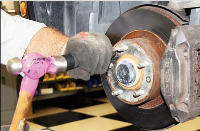
**Sequence 2:** Break loose the hat locator screws using an impact screw driver. Then remove the screws.
