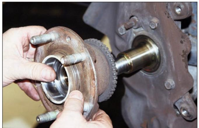
**Sequence 18:** After the spindle nut is removed, slide off the hub assembly and save for reinstallation later.
