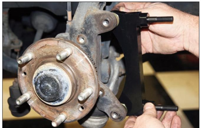
**Sequence 24:** Attach the Wilwood caliper mounting bracket to the OEM mounting ears from the back side. Temporarily tighten the mounting bolts. **NOTE:** The bracket must fit squarely against the mounting ears. Inspect for interference from casting irregularities, burrs, etc. Grind as necessary. Do not Loctite at this time.
