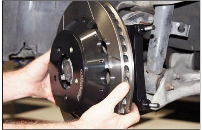
**Sequence 28:** Install the hat/rotor assembly over the studs on the hub assembly. **NOTE:** The hat/rotor must fit flush against the axle hub flange or excessive rotor run out may result.
