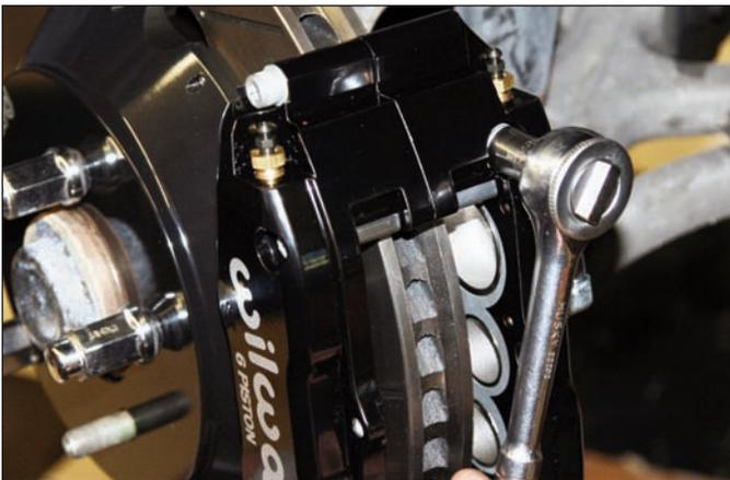
**Sequence 33:** Secure the caliper with washer and locknut, temporarily tighten. View the rotor through the top opening of the caliper. The rotor should be centered in the caliper. If not, adjust by adding or subtracting shims between the bracket and the mounting ears. Once the caliper alignment is correct, remove the bracket bolts one at a time and apply red *Loctite*® 271 to the threads and torque to manufacturer's specifications.
