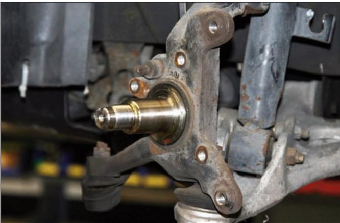
**Sequence 20:** Clean and remove any nicks or burrs on the spindle as well as the OEM caliper mounting ears that may interfere with the installation of the new Wilwood caliper mounting bracket.
