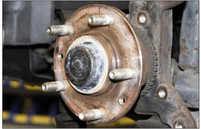
**Sequence 22:** Reinstalled the OEM dust cap.
