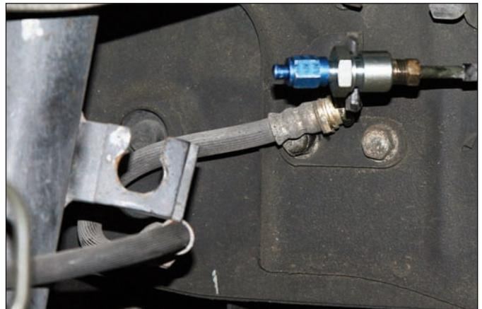
**Sequence 6:** Using a fitting from the new Wilwood flexline hose kit, P/N 220-7010 install the fitting on the end of the hard line. Temporarily cap or plug the fitting to keep fluid from draining out of the line while continuing with the installation.
