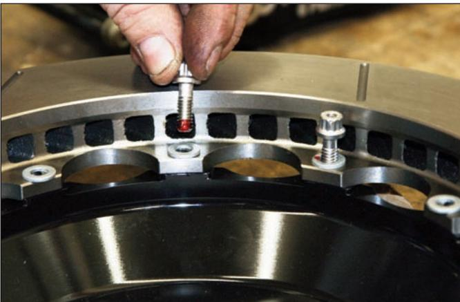
**Sequence 27:** Place one flat washer over each hole on the rotor mounting tabs. Coat the mounting bolts with red *Loctite*® 271 and slide through the washer and thread into the hat. Using an alternating sequence, torque bolts to 155 in-lbs.
