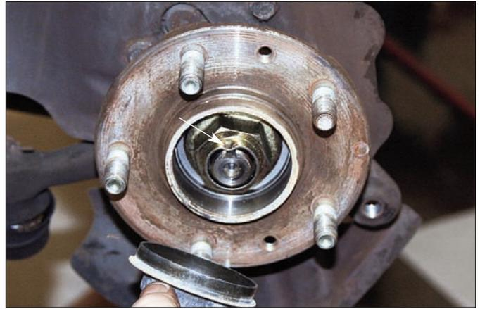
**Sequence 16:** After the dust cap is removed, the crimped over area of the spindle nut needs to be straightened so that it can be removed (arrow).
