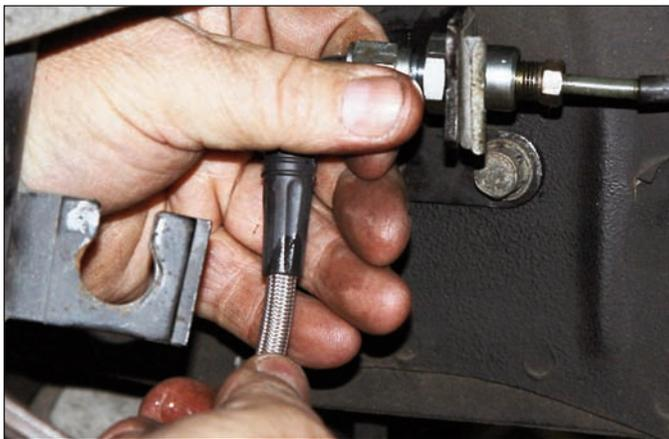
**Sequence 38:** Connect the other end of the flexline to the fitting at the brake hard line. Secure line as necessary to prevent contact with moving suspension, brake, or wheel components. Bleed the system referring to the additional information in the data sheet as necessary for proper bleeding instructions.
