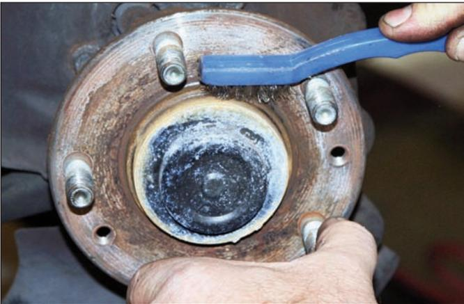
**Sequence 14:** Clean the hub assembly with a wire brush and remove any nicks, burrs, or grease that may interfere with installation of the new brake components.
