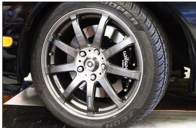
**Sequence 39:** Install the wheel and torque the lug nuts to manufacturer's specification. Bed in the brake pads and rotor in a safe location before general use driving.
