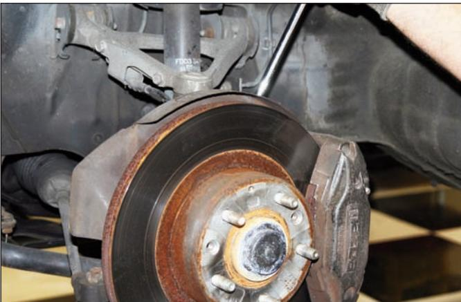
**Sequence 3:** Using a breaker bar and socket, break loose the caliper mounting bolts from the back side. Do not completely remove at this time.
