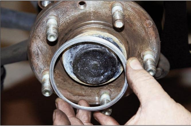
**Sequence 25:** Install the rotor registration adapter over the hub dust cap against the hub face with the larger O.D. facing inward toward the hub face.
