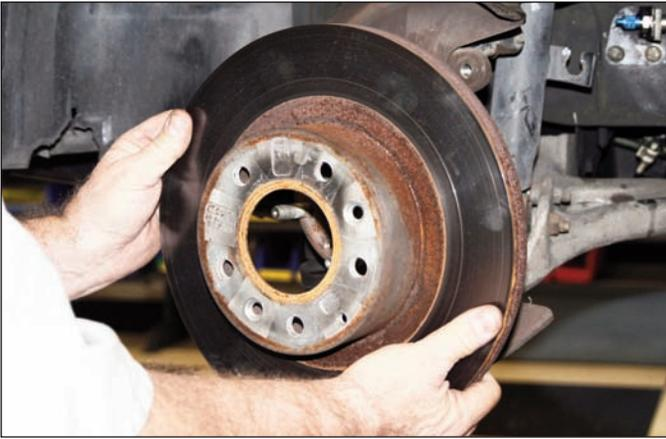
**Sequence 13:** Slide off the rotor from the hub. If it is stuck, it may be necessary to hit it a few times with a rubber mallet to break loose.
