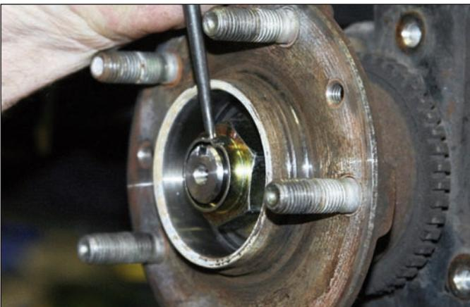
**Sequence 21:** Slide the saved hub assembly onto the spindle and secure with spindle nut. Torque to OEM specifications. Follow the OEM recommendations regarding the reuse of spindle nuts. It may be necessary to source new spindle nuts. Using a screw driver, crimp over the flange of the spindle nut to keep it from unscrewing.
