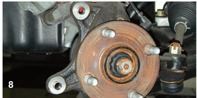
The rotor was removed so that the Caliper bracket could be connected to the original mounting ears. The holes in the ears are larger than necessary, so here sleeves were installed to get the holes down to the bolt size.
