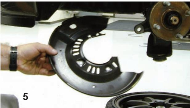
After the cuts were made, the dust shield could be removed from the hub assembly.
