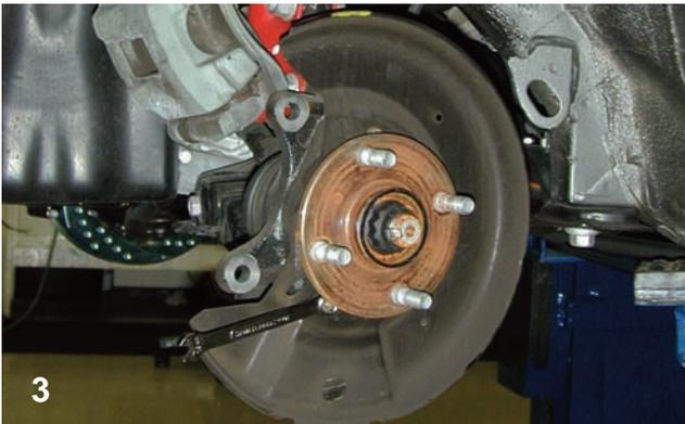
After the rotor was removed from the assembly, you can easily see the two mounting ears that will be used to connect the Wilwood caliper mount.
