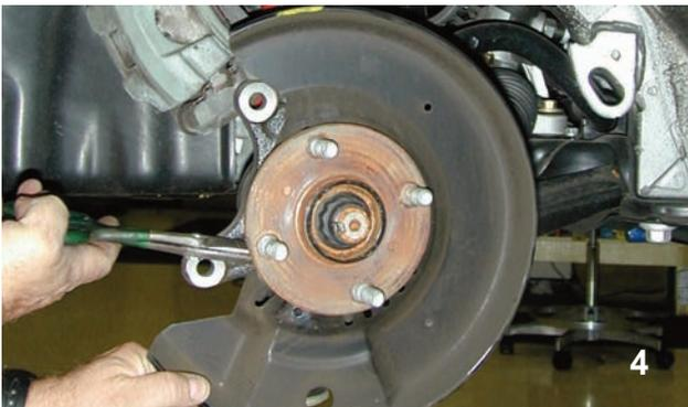
The small bolts securing the dust shield were removed and then the dust shield was cut with metal shears to remove it from the hub assembly.
