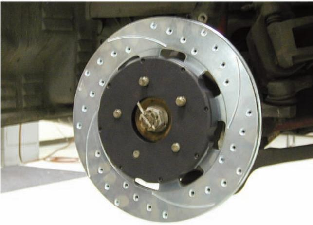
Using the bolts included in the kit, the caliper was mounted to the hat. The bolts were coated with Loctite 271 and then the hat was joined to the rotor by tightening the bolts. After all of the bolts are finger tight, they should be tightened in an alternating sequence to 144 in-lbs using an inch-pound torque wrench. After the caliper was assembled it was installed on the Eclipse hub assembly.
