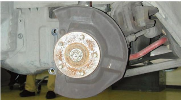
After the caliper was removed, you can see the two caliper mounting ears protruding past the dust shield.
