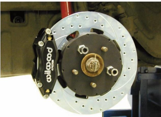
Two lug nuts were used to tighten the rotor to the hub assembly, then the caliper was installed on the bracket using the 5/4-inch thick washer and the spacer on each stud. The caliper was then mounted and the small flat washer and self-locking hex nut were installed.
