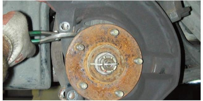
The two bolts that secure the dust shield to the hub were removed and since the dust shield will no longer be needed it was cut with hand shears to remove it from the assembly. The dust shield metal could also be cut with a three-inch cut-off wheel.
