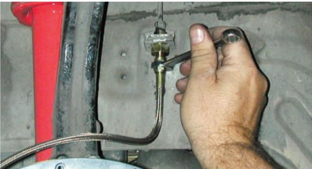
The fitting that was used was connected to the inner fender bracket with a brake line clip. Here the Wilwood braided steel line is being connected to the fitting.
