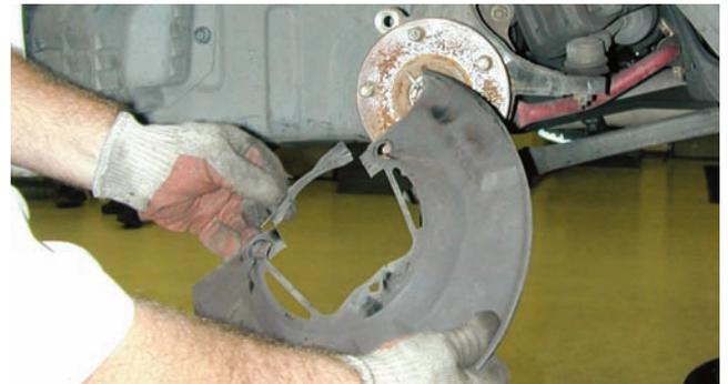
This small section of metal was cut away from the dust shield to remove it from the assembly rather than removing the hub assembly.
