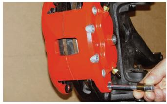
This view shows how the sleeve fits over the bolt and it will fit into the caliper body. The bolts screw in from the backside and the threads are close to the head of the bolt.
