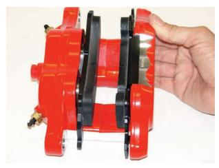
The pads fit into the caliper as seen here. The pads on the piston side are held in place by the bolts while the other side is held in place by the metal tab that fits into the caliper body.
