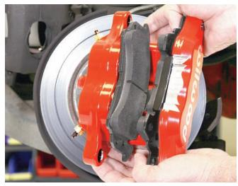
Before the caliper was installed the pads were loaded into the unit as seen here. The brake pads load into the caliper from the bottom as shown. We installed the Wilwood kit in this installation and it came with new pads, however the old pads could be retained and reused. If using old pads the retainer clip will have to be discarded.
