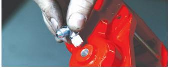
The caliper inlet fitting threads were wrapped with Teflon tape and then the fitting was installed in the side of the caliper. The 90-degree inlet fitting was rotated until it faced the upper bleed nipple.
