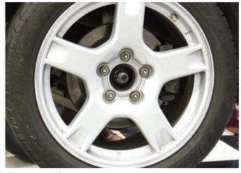
The original Corvette hubcaps were removed to access the lug nuts. Using the correct size socket and an impact gun, the lug nuts were disconnected and the wheels were removed.
