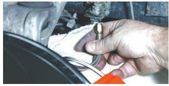
To finish off the front brakes, the braided steel flex line coming from the caliper inlet fitting is connected to the hard-line that rests in the chassis mounted bracket.
