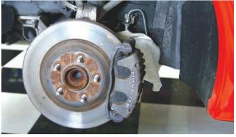
The car was raised using the floor jack and then jack stands were placed underneath in a safe Corvette specified place. The two tires that were still resting on the ground were chocked to keep the car from moving. The wheels and tires were removed and here you can see the original Corvette caliper and rotor assembly.
