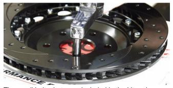
The small bolts that were included in the kit and were previously coated with Loctite 271 were used to connect the rotor to the hat assembly. The bolts were tightened in an alternating sequence to 85 in-lbs. After the bolts were tight, they were safety wired following the diagram in the instruction sheet.
