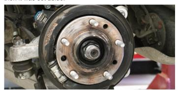
The rotor face was tapped on the backside to release it from the centering ring. When it was loose it was removed from the assembly. If you look closely you can see the two mounting ears that will be used to secure the Wilwood caliper bracket.
