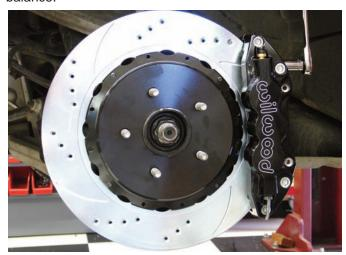
The rotor was attached to the bracket and the centering was checked and achieved. After the centering was perfect, the caliper mounting bolts were coated with Loctite 271 and were tightened to 65 ft-lbs using a torque wrench.
