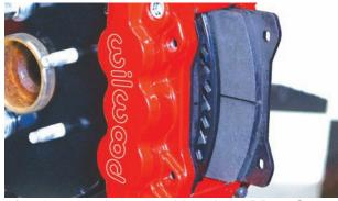
After the centering was achieved, the BP-10 Smart Pads were installed in the caliper and then the two retaining clips and snap rings secured the pads.
