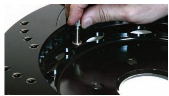
Here the bolts are being installed and they were tightened in an alternating sequence.
