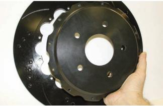
The hat assembly is being lined up with the tabs on the rotor. This hat is designed to work with the original Corvette internal parking brake assembly.
