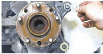
Two shims were placed on both of the mounting bolts before the bracket was installed. This will be a starting point to get the caliper centered over the rotor. This may be perfect the first time, but shims can be added or subtracted to get the caliper centered over the rotor.
