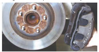
The two caliper mounting bolts were disconnected and then the rotor was lifted away from the brackets. The original brake line can be removed from the chassis bracket and the line should be capped to prevent fluid from leaking out.
