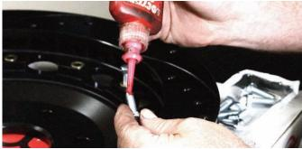
Before the assembly could go any further, the hat to rotor connection was made. The small bolts that make the connection were coated with Loctite 271.
