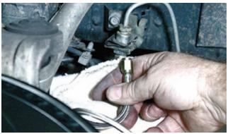
The Wilwood Engineering Flexline was routed from the caliper inlet fitting to the rear frame bracket that secures the original hard line. Here the two are being attached.
