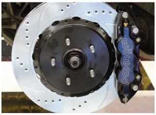
The brake pads were installed and secured with the center bridge pad retaining bolts. Here is the rear brake assembly ready for action. This system is great on the street but it is also track ready.
