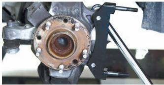
Using the two mounting bolts that were loaded with two shims, the Wilwood caliper bracket was installed and it was tightened down. After the perfect centering is accomplished these bolts will be coated with Loctite 271 and they will be tightened to 65 ft-lbs using a foot-pound torque wrench.
