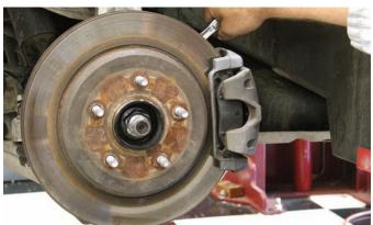
Using a socket wrench and the appropriate size socket, the two bolts that secure the caliper to the upright bracket were disconnected and removed.
