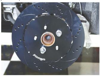
The assembled rotor was installed on the hub assembly. The rotor was secured with two temporary washers and lug nuts to allow the caliper to rotor centering process to be done.
