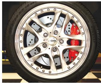
The wheels were installed and the brakes were bedded in. The bedding process removed the E-coat from the rotor surface leaving a nice silver rotor face while the rest of the rotor remains coated and protected.
