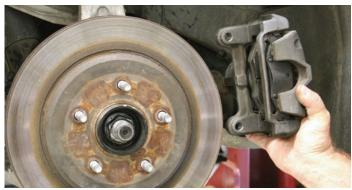
After the bolts were removed from the caliper bracket, the loose caliper was removed from the bracket assembly and then it was set aside.
