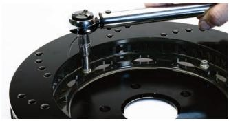
After all of the bolts were installed, they were tightened in an alternating sequence to 85 in-lbs using an inchpound torque wrench.
