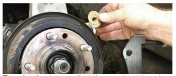
The caliper bracket mounting bolts were placed through the ears and then they were loaded with two shims per bolt.
