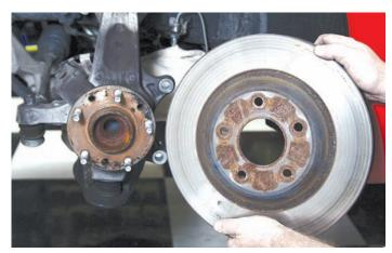
After the caliper was disconnected and shelved, the rotor could be removed from the hub assembly.
