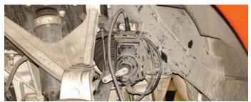
In order to access the OEM hard to hose connector, the two bolts that secure the OEM Automatic Suspension Control Module to the fender well were removed and the unit was moved out of the way.
