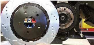
All of the Wilwood rotors are currently E-coated black for protection but in this photo a rotor that was zinc coated was used. This rotor is drilled and slotted for a nice appearance and to displace heat and brake dust.
