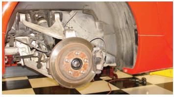
Here is the Corvette independent rear suspension system complete with the stock brake system. The newer Corvettes are much more sophisticated than they were in the past.
