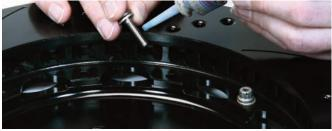
Now it is time to mount the hat to the rotor. The bolts and hat threads must be clean and free of oil or other contaminants. Loctite 271 was applied on the threads in preparation for installing them in the rotor to hat connections.
