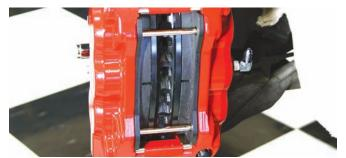
After the centering was achieved, the BP-10 Smart Pads were installed in the caliper and then the two retaining clips and snap rings secured the pads.
