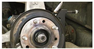
Here is the caliper bracket after it was secured to the original mounting ears. The bolts should be tight but just enough to check the rotor to caliper centering. After the centering is found, the bolts should be coated with Loctite 271 and tightened to 65 ft-lbs using a torque wrench.
