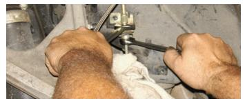
With the Automatic Suspension Control Module out of the way, the bracket that secured the hard line to hose line connection was easy to access. Using a line wrench, the two lines were disconnected. This is the same location where the Wilwood rear Flexlines will be connected after the brakes are installed.
