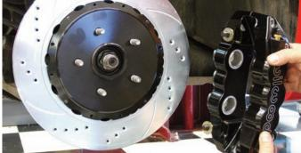
The rotor was attached to the rear hub assembly and here the caliper is ready to be installed. Notice that the rotor bolts are loaded with a two 0.035-inch shim washers per bolt. The calipers were tightened with a washer and self-locking nut per stud. Four piston calipers are used in the rear and they provide a good front to rear balance.
