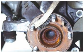
The face of the hub assembly and the lug nut threads were cleaned with a wire brush. Any debris left on the hub can keep the rotor from properly seating, resulting in runout. Here you can also see the original caliper mounting ears where the new caliper bracket will be connected.
