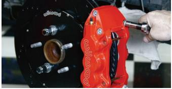
The caliper was installed on the studs and it was tightened using a socket wrench. Now the caliper to rotor centering process was done to make sure rotor is centered in the caliper. The caliper can be moved inside or outside just a little by adding or subtracting shims. After the center position was achieved, the caliper mounting bolts were coated with Loctite 271 and were tightened to 85 in-lbs.
