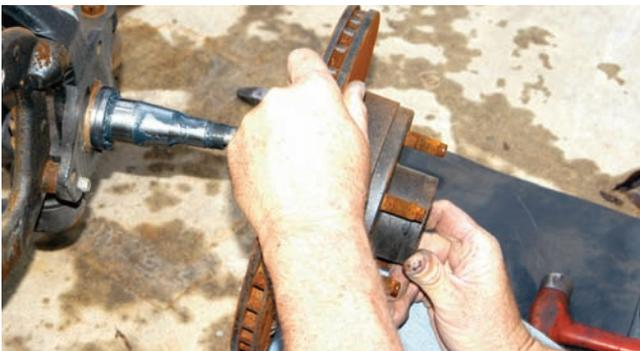
The one-piece 11-inch rotor was removed from the spindle. Save the rotor and caliper because they could be used on another car or sold at the local automotive swap meet.
