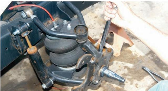
The two bolts securing the caliper bracket to the spindle were removed. These will be very tight so you might want to loosen them up with a little WD40 or JB80 penetrant.
