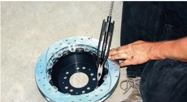
The bolts are designed with safety wire holes to make sure they don't back out. Here the safety wire is being connected.
