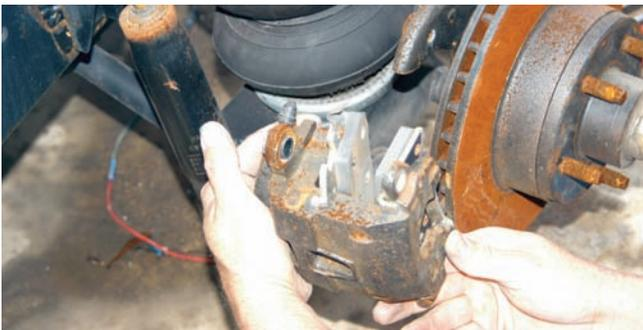
The calipers are being removed from the brackets. Remember to disconnect the brake lines before this is done.
