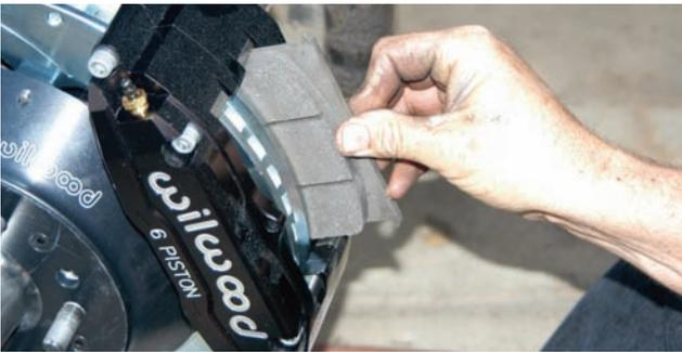
The pads are installed from the top making the installation very easy. They were dropped in place after the alignment was perfect.
