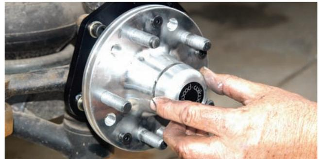
After the hub was installed, it can be finished off with the screw-on hub cover.
