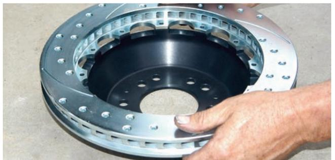
Wilwood uses a two-piece rotor that features an aluminum hat that connects to the steel rotor. One reason for the two-piece arrangement is the large 13-inch rotor can be adapted to hats for a wide variety of applications. This hat has holes for the Chevy and Ford lug patterns.
