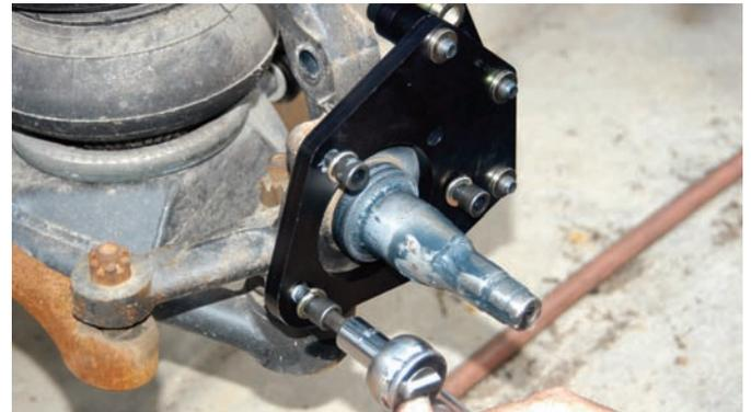
The brackets were installed on the Mustang II-style spindles with the three high-strength Allen bolts and the machine washers that came in the kit.
