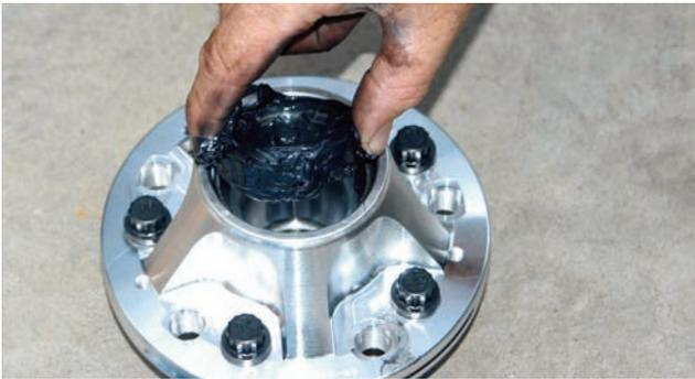
The greased bearing was installed in the rear of the hub making sure it was facing in the correct direction. The bearing race comes installed in the hub assembly.
