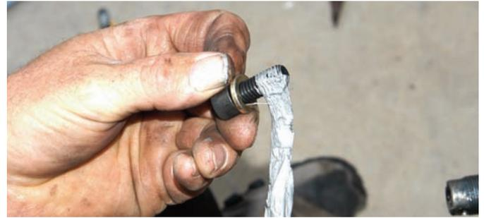
The Wilwood caliper bracket was installed at this point, but before it was, the mounting bolts were coated with Loctite Anti Seize.
