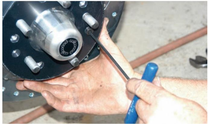
There are three small screws that secure the rotor to the hub assembly. These small screws do not take the braking force, the lug nuts does that.
