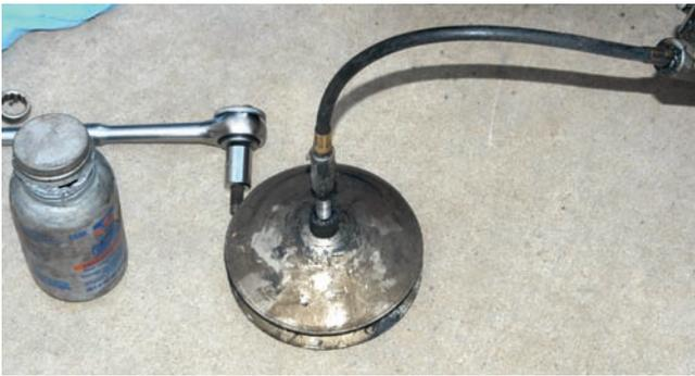
The large rear wheel bearings are installed first. Since all of the bearings have to be packed with high temperature disc brake bearing grease, all four bearings were packed using this bearing packer.
