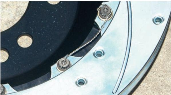
Here are the bolts with the safety wire installed. All of the bolts will need safety wire but you can install the wire to two or more bolts at a time. The only special tool you will need is a safety wire pliers.
