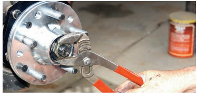
After the hub was on the spindle and the bearing was loaded, the large washer was installed followed by the large spindle nut. The nut was tightened with channel lock pliers but it could also be done with a large jaw Crescent wrench. The nut should be snug but not too tight, because an over tight nut will burn out the bearings.
