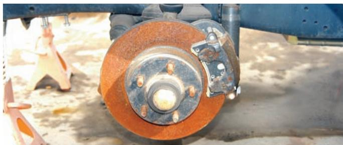
This '34 Ford was equipped with an Art Morrison independent front suspension system with airbags and GM disc brakes. The GM brakes are effective in most situations, but since this rod is powered with a 502 horsepower 502ci Chevy big-block engine, the owner wanted superior stopping power.
