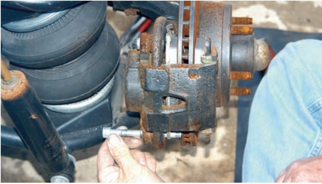
The old system was removed first and that began by disconnecting the two large Allen bolts that secure the calipers to the brackets.
