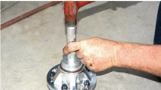
The kit comes with a grease seal, so it was installed with this seal installation tool. A few good whacks and the seal bottoms out in the hub.
