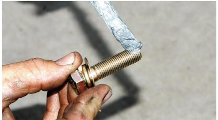
After the rotor was secured to the hub, the calipers were installed. Before they were installed the mounting bolts were coated with Loctite Anti Seize. Notice that the bolts are also equipped with a lock washer and a flat washer.
