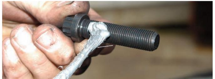
This system uses a hub and hat assembly so the hub has to be installed first. The procedure began by coating the lug nuts with Loctite Anti Seize.
