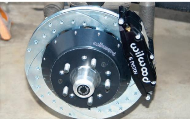
Here is the finished brake assembly with the large 13-inch rotor and six-piston caliper. It will work great to stop this powerful Chevy street rod and it is also a very attractive addition.
