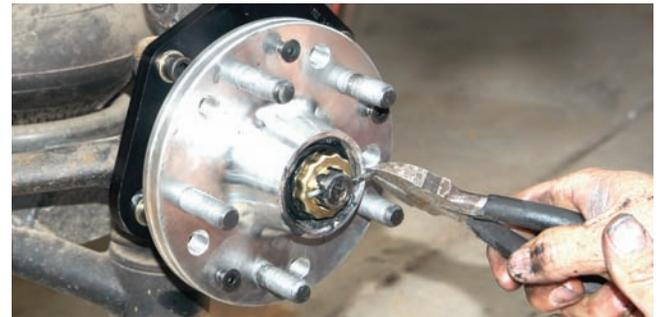
Since the nut can't be torqued down to keep it tight, it is necessary to keep it in place another way. Here the nut is equipped with a castle-style cap that works in conjunction with a cotter key.
