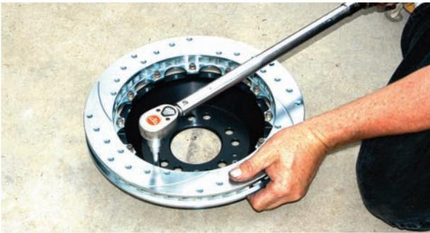
After the holes were lined up, the rotor was installed to the hat assembly with the high strength 1/4-inch Allen bolts supplied in the kit. The rotor bolts were tightened to 85 in-lbs using an inch-pound torque wrench.
