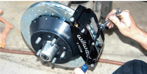
After the brake pads were installed, the bridge bolt and tube were screwed back in place. It is important to make sure the connection is tight.
