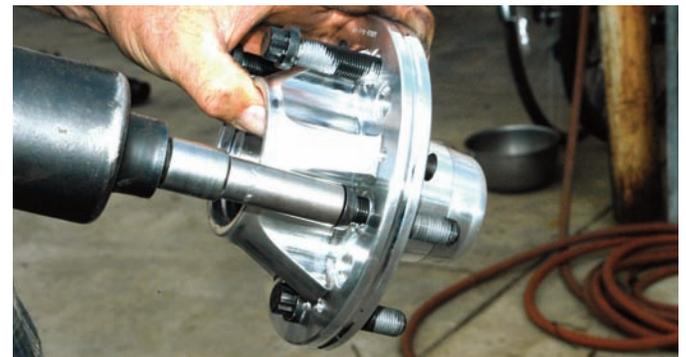
There are two lug patterns in the hub assembly so the lug nuts have to be installed in the one that applies to your vehicle's wheels. This car is running a Ford 5 on 4 1/2-inch lug spacing. The best way to install the lug nuts is with an impact gun because it will get them tight enough to stay in place. If you try to do this with a wrench, the lugs won't be tight enough and will back out later. After using the impact gun, the lug nuts should be tightened to 77 ft-lbs using a torque wrench.
