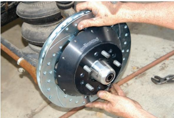
After the safety wire job was completed, the large 13-inch rotor could be installed on the hub.
