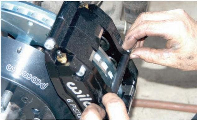
The calipers feature a bridge bolt and aluminum tube to keep the pads in place. Here the bolt is being removed so that the pads can be installed.
