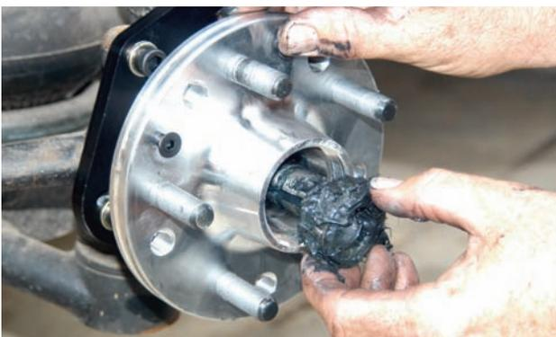
The hub was installed on the spindle and then the small bearing was installed.
