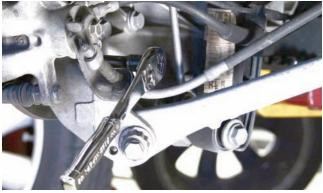
The bolts that fasten the caliper to the bracket were removed from the backside of the assembly as seen here.
