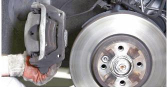
After the bolts were disconnected, the cast iron caliper was removed from the brake assembly. The new brake caliper is much lighter than the old caliper.
