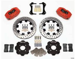
The Wilwood part number 140-8528 front disc brake kit comes complete with the rotors, hats, DynaPro calipers, pads, caliper brackets and all of the hardware required to finish the installation. The kit ordered features red calipers and the slotted and cross-drilled rotors.
