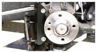
The bracket should be tight to check the rotor to caliper centering. It should be centered but if it is not, shims can be added or subtracted to get it perfect. After the centering was perfect the bracket bolts were coated with Loctite 271 and then they were tightened to 75 ft-lbs.
