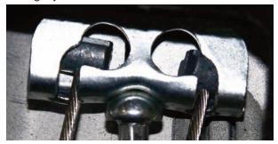
The console was removed to access the handbrake cable equalizer with two cables going toward the rear. The two cables were removed from the equalizer and they were pushed toward the rear. The OEM cable end clips are hidden at the very rear of the tunnel and hidden under the rearward brace. Using a four-inch long metal tube, it was forcefully placed into each clip and then the cable was twisted and pulled out of the holes.
