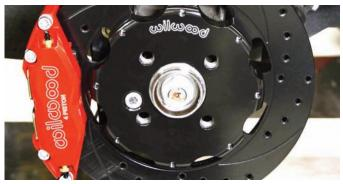
The finished brake assembly is looking good with the bright red caliper and black E-coated rotor. This system will improve the Mini braking, plus it looks nice doing it.
