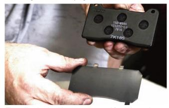
The adhesive backing was removed from the antisqueal plate and then it was attached to the rear side of the brake pad. The tabs were bent over the pad baking plate to keep them in place.
