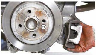
After the bolts were disconnected, the caliper was removed from the bracket and the car.
