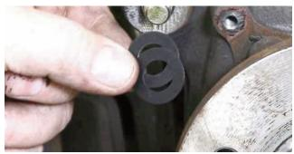
The bolts were installed into the original caliper mounting holes and two shims were installed.
