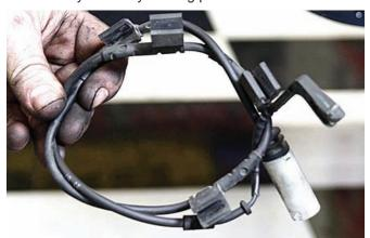
The brake wear sensor line was wrapped up and it can be installed in an inconspicuous place while connected in the car. If the brake sensor line is removed completely, the brake wear dash warning light will remain on.
