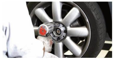
Using a floor jack, the front of the Mini was raised and was placed on jack stands. The hubcaps were removed to access the lug bolts. Using the proper size socket and an impact gun the lug bolts were disconnected and the wheels and tires were removed.
