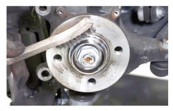
Before going any further, a wire brush was used to clean the grease and grime away from the hat locator on the hub.
