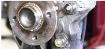
The caliper bracket bolts to the same location the original caliper bolted to. Here you can see the bolts in the holes and they will be used with a two shims per bolt.
