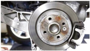
Here is a look at the factory disc brake setup that connects to a hub assembly that rides on a large aluminum lower control arm.
