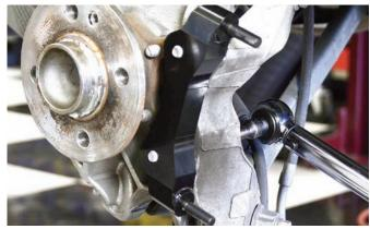
Here is the caliper bracket after the bolts were installed and tightened. The caliper to rotor centering was perfect before the final installation. After it was determine that the centering was perfect, the bolts were coated with Loctite 271 and they were tightened to 22 ft-lbs using a torque wrench.
