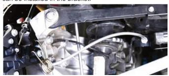
Here is the Wilwood part number 220-10879 braided steel Flexline running from the caliper to the bracket holding the steel line and adapter fitting. The line was routed away from any moving parts.
