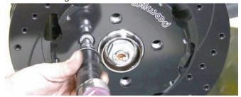
The rotor was attached to the hub assembly using the same torx bolt that fastened the original rotor. The impact screwdriver is reversible so a few whacks of the hammer got the bolt very tight.
