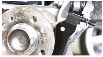
Before the caliper was installed, the bracket studs were loaded with two shims per stud.
