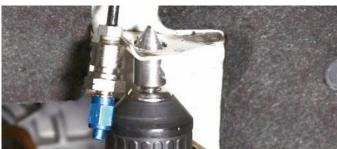
After the original line was removed the bracket was drilled out just a little so that the adapter fitting seen here can be installed in the bracket.
