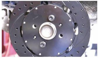
The rotor was placed on the hub assembly and then it was tightened with two lug bolts.
