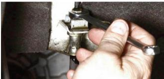
The old brake hose was removed and the new Wilwood part number 220-8491 was installed remembering to install the rubber grommet that were removed from the original hose. The hole in the bracket will have to be enlarged to hold the fitting used to adapt the Wilwood Flexline to the original steel line.
