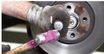
The torx bolt that secures the rotor to the hub was very tight, so it was loosened with an impact screwdriver. The bolts were retained because they will be used to fasten the new rotors.
