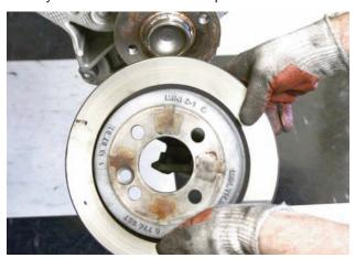
After the bolt was disconnected, the rotor was removed from the hub assembly. If the rotor sticks to the centering ring, a few taps with a rubber mallet will loosen the connection.
