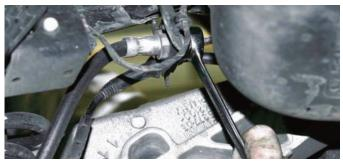
The line that was just connected to the caliper fitting was routed to this frame bracket. There is a special connection that adapts the braided line to the original steel line. The original flexible line was disconnected from the steel line first and then the bracket was modified for the new adapter fitting.
