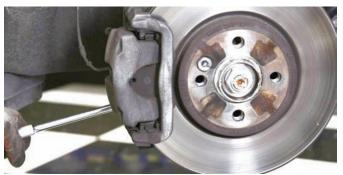
Using a breaker bar and the correct size socket, the caliper bolts were disconnected from the front hub assembly.
