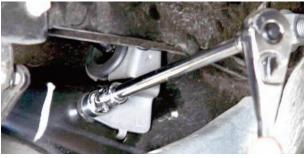
The bolts fastening the cable brackets on the rear suspension arms were also removed so they can be slightly modified.
