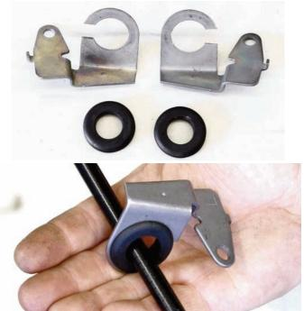
The mounting brackets that were previously removed were modified so the new lines could be run through. Using two grommets, they were placed over the line and were pressed into the small brackets as seen here. After the lines were in place, the small brackets were bolted back on the control arms.
