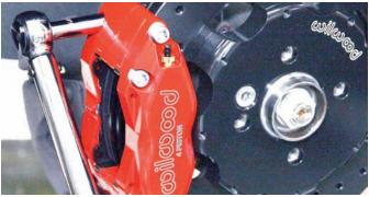
The caliper was placed on the caliper bracket and then the washers and locknuts were installed. Make sure the rotor is centered in the caliper, and when it is, the studs were lightly oiled and the mounting nuts were tightened to 30 ft-lbs using a torque wrench.
