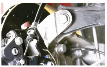
The lines were run forward and here is how they were attached to the master cylinder lever.
