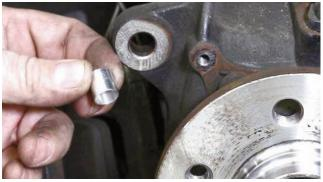
The original caliper mounting holes are rather large, so bushings are used in the top and bottom hole to downsize the holes.
