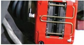
Here is a close look at the Quick-clip pad retainer that makes pad changes easy. Here you can also see that the rotor is centered between the pads.
