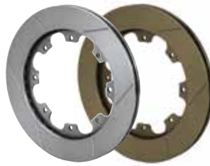
GT 36 Curved Vane 160-12285 (R) 160-12286 (L) 160-12285-B (R) 160-12286-B (L) 0.81" Width 11.75" Diameter
