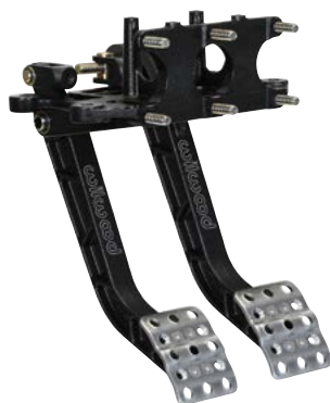
340-11299 6.25:1 340-13835 5.1:1 340-13836 6.25:1/5.1:1 Reverse Swing Mount Brake and Clutch Pedal
