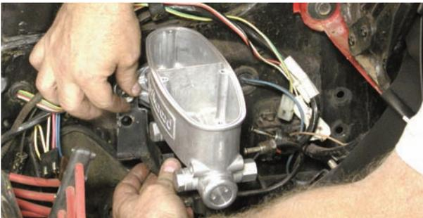
The old master cylinder was removed and the new one was bolted in place. The Wilwood part number 260-9439-P master cylinder has slotted mounting holes so it will fit perfectly in many locations such as this Camaro where it bolts right on.
