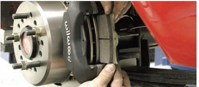
The rotor was installed and it was bolted to the axle. The caliper was connected to the bracket and then the caliper to rotor centering was determined. After the caliper was in alignment, the bolts were coated with Loctite 271 and then they were installed and tightened to 30 ft-lbs. After the caliper was centered, the BP-10 Smart Pads were installed.
