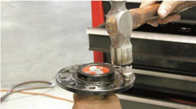
Wilwood hats center on 1/2-inch studs and Chevy uses 7/16-inch studs. You will have to take the axles to a machine shop and have the lug holes drilled and tapped for fine thread 1/2-inch lug studs.
