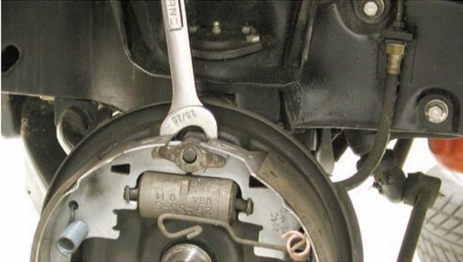
Using a large 15/16-inch wrench, the center bolt was removed from the backing plate and spindle.
