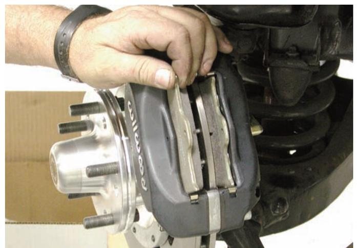
The BP-10 Smart Pads were installed into the rotors from the top. They should fit in without any binding and should seat all the way in. The Smart Pads are perfect for normal driving around town and on the highway.
