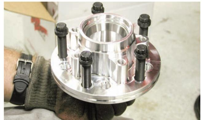
Using the correct Chevy 5 on 4 3/4-inch spacing, the lugs were installed into the aluminum hub assembly. The lug studs were tightened to 77 ft-lbs.
