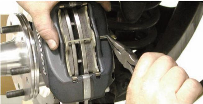
The brake pads are secured with a long cotter key. The ends were bent enough to hold the key in place but not too much because the key will have to be used again when the pads are replaced in the future.
