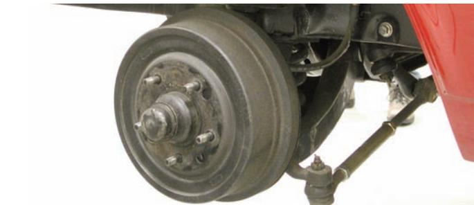
This '67 Camaro came from the factory with standard four-wheel drum brakes. Disc brakes were optional in 1967 and they were primitive. We are updating this Camaro with a Wilwood part number 140-2285-B disc brake kit that can be installed on disc or drum brake spindles.
