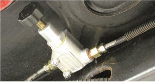
Since this is an entirely new brake system a part number 260-8419 proportioning valve was installed to the rear brake lines under the Camaro. The knob was positioned toward the outside of the car for easy access. This valve can be used to set the front to rear brake bias.
