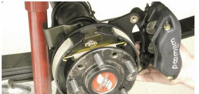
The caliper was held up to the bracket to check the bolt spacing. Everything was looking good but the caliper couldn't be installed until the rotor was connected.
