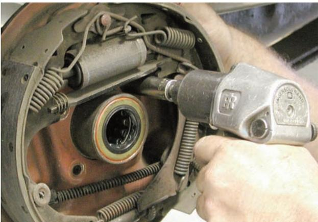
The four backing plate to axle flange bolts were removed using an impact gun and an open-end wrench. After the bolts were disconnected the backing plate was removed from the axle.
