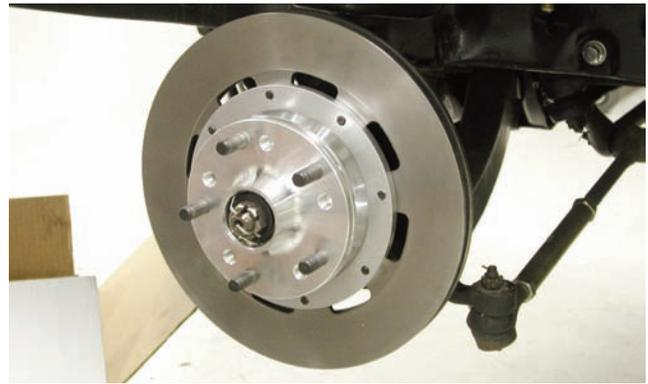
The rotor was placed on the spindle, the small bearing was installed into the front of the rotor, the washer was placed back on and then the large nut was screwed onto the spindle end. This is a critical connection so the nut was tightened snug but not over tight because that could cause premature bearing failure. After the nut was snug the castle portion was aligned with the hole in the spindle end and a large cotter key was installed to keep the nut in place.
