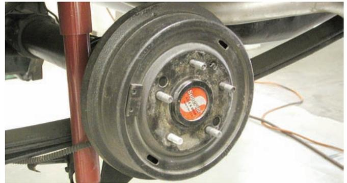
The front wheels were bolted onto the disc brakes and the front of the car was lowered so the rear of the Camaro could be elevated. This Camaro features a strong running small-block Chevy engine so it is equipped with a 12-bolt Chevy differential. Drum brakes are used at the rear so Wilwood rear disc brakes will get this Camaro stopping efficiently.
