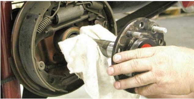
The axles were carefully removed from the housing making sure you note which side they came out of. Many differentials have a short and a long axle.
