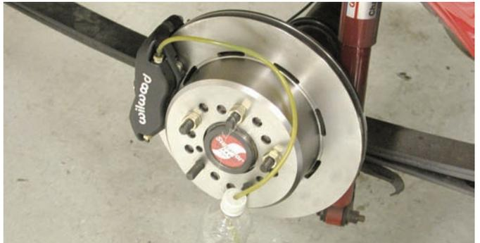
Here is the finished rear brake assembly and it certainly will be a nice performance addition to this '67 Camaro. After the bleeding procedure is finished the brakes will have to be bedded following the procedure outlined on the instruction sheet.
