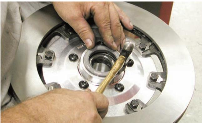
The hubs come complete with the inner and outer spindle bearings, so before they were installed, they were packed with high temperature disc brake bearing grease. The large bearing was placed into the rotor hub and then the grease seal was installed.
