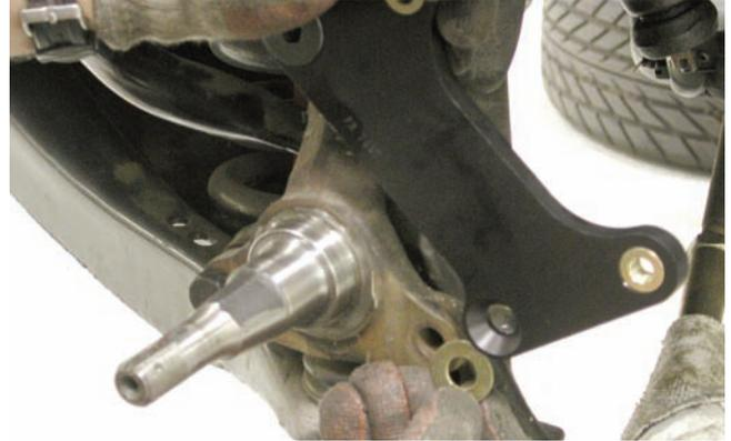
The caliper bracket was installed using the two spacers in the kit. The large spacer and a washer are used at the top connection and a small spacer and a washer are used at the lower connection.
