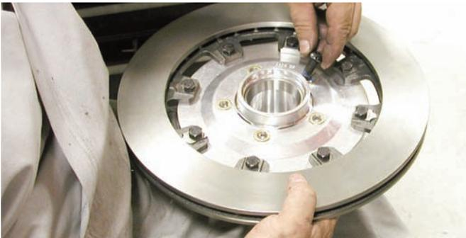
The hub assembly was connected to the rotor adapter plate using the bolts supplied in the kit. Using a torque wrench, the bolts were tightened to 22 ft-lbs and then they were safety wired.
