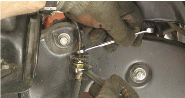
Before the backing plate could be removed, the brake hose had to be disconnected from the steel line. Here the connection is being disconnected with an open-end wrench and a line wrench.
