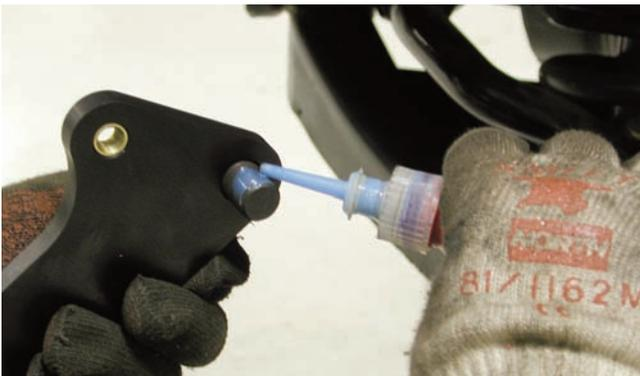
After the backing plate was removed, the caliper bracket could be installed. The bolts were coated with Loctite 271 before installation.
