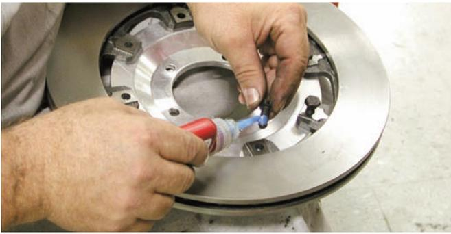
The rotor adapter plate was connected to the rotor using the bolts supplied in the kit. Before the bolts were installed they were coated with Loctite 271.
