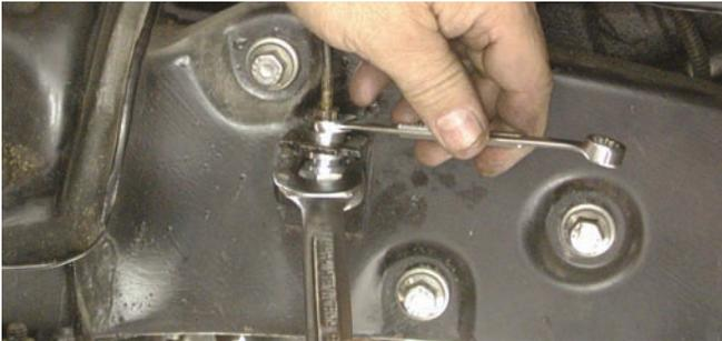
The Wilwood Flexline was connected to the original steel line using an open-end wrench. The Flexline was secured with an open-end wrench and the steel line was tightened with a line wrench after the initial connection was made.
