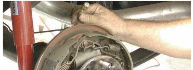
Using a line wrench, the original steel lines were disconnected from the wheel cylinders on both sides of the car.
