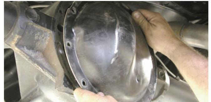
The axles have to be removed from the differential so the differential cover was removed to access the C-clips. A drip pan was placed under the axle, the cover bolts were disconnected and then the cover was carefully lifted and removed from the axle. Before this is done, it would be advisable to have another pan gasket and some silicone ready for installation.
