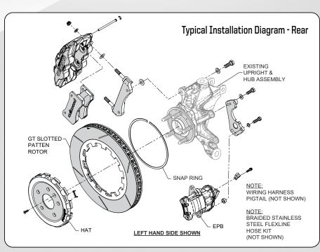
AERO4/ST Rear Kits GT Slotted Rotor, Burnished, Electric Parking Brake
