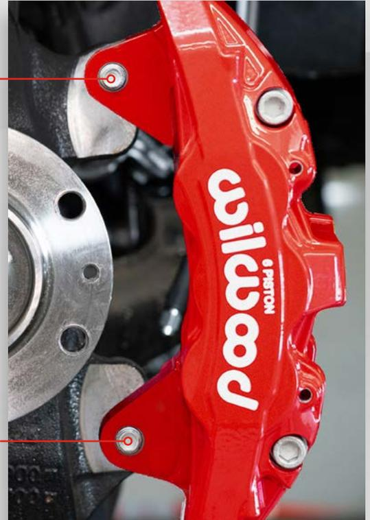
Caliper Mounts Directly to Factory Spindle
