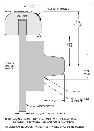
Figure 2. Wheel Clearance Diagram
