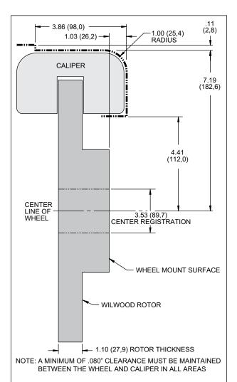
Figure 2. Wheel Clearance Diagram
