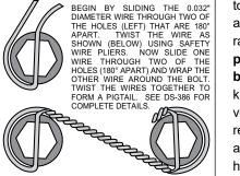
Figure 3. Safety Wire Diagram
