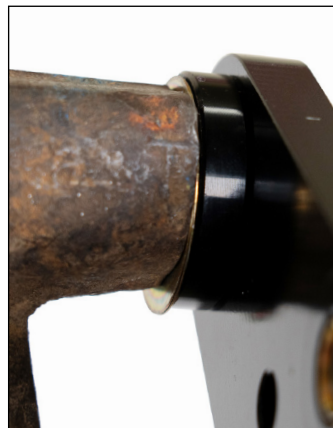
Photo 2 Spacer for drum spindle (.250")
