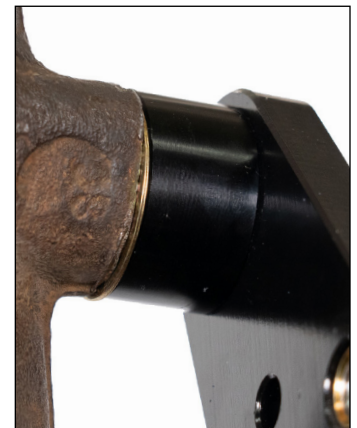
Photo 3 Spacer for disc spindle (.700")
