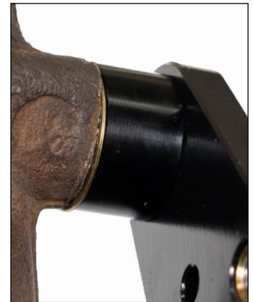
Photo 3 Spacer for disc spindle (.700")
