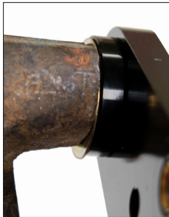
Photo 2 Spacer for drum spindle (.250")
