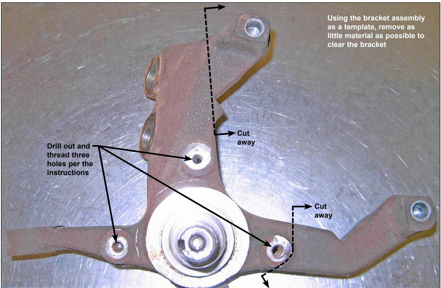
Photo 1. Typical Steering Arm / Spindle Modifications
