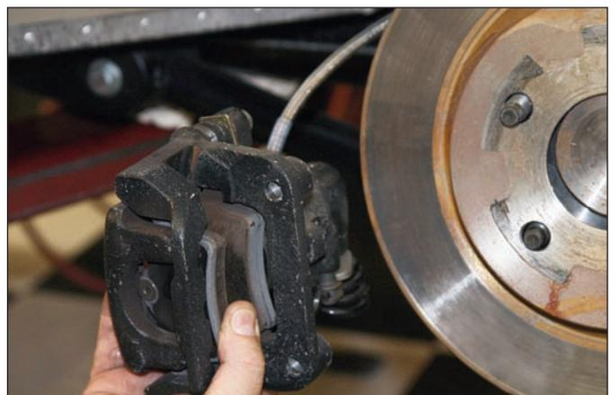
**Sequence 5:** Disconnect the parking brake cable. Lift off the caliper and keep the OEM brake line hose in the vertical position to avoid spilling brake fluid that remains in the hose.
