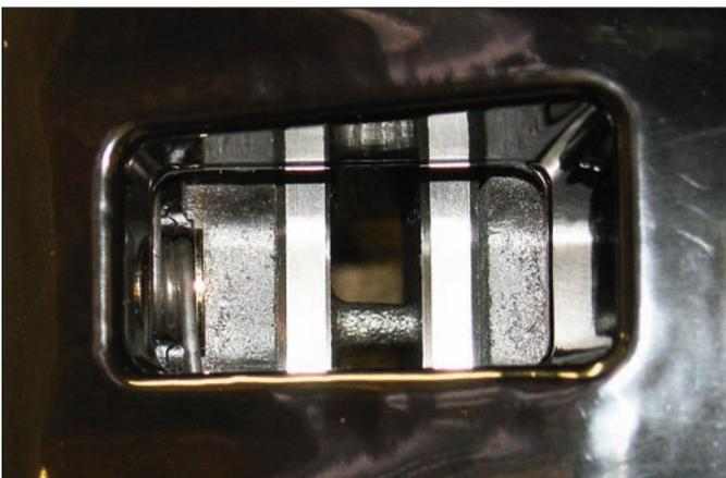
**Sequence 20:** View the rotor through the top opening of the caliper. The rotor should be centered in the caliper. If not, adjust by adding or subtracting shims between the caliper mounting bracket and the flat bracket. Once the caliper alignment is correct, remove the bracket bolts one at a time and apply red *Loctite*® 271 to the threads and torque to 22 ft-lb.
