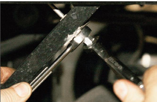
**Sequence 3:** Disconnect the OEM brake fluid hose where it connects to the brake hard line. Temporarily cap (not included) the line to minimize fluid loss.
