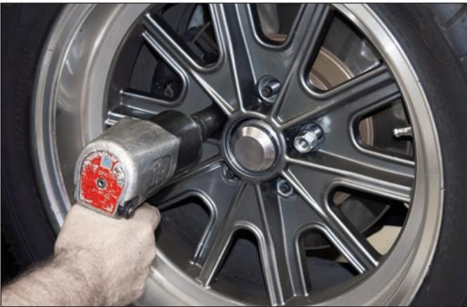
**Sequence 2:** Hiding behind the knock-off is the lug nuts, remove those and lift off the wheel.
