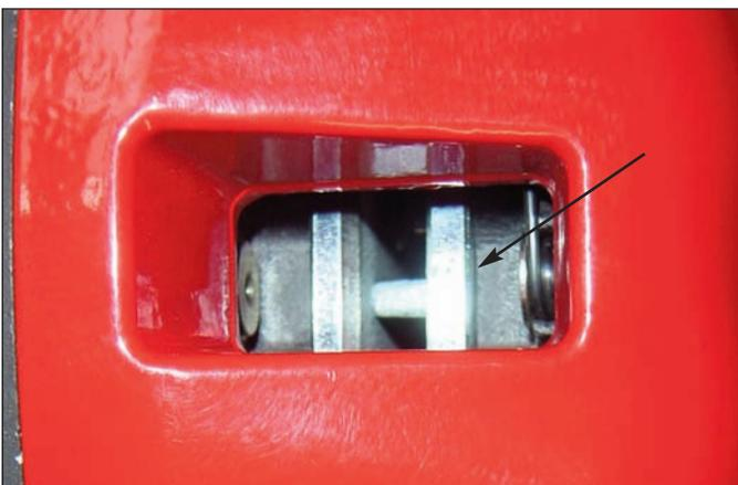
**Sequence 21:** Check that the top of the brake pad is flush with the outside diameter of the rotor (arrow). If not, adjust by adding or subtracting shims between the bracket and the caliper. After bleeding (sequence 22), reinstall caliper and torque caliper nuts to 35 ft-lb.
