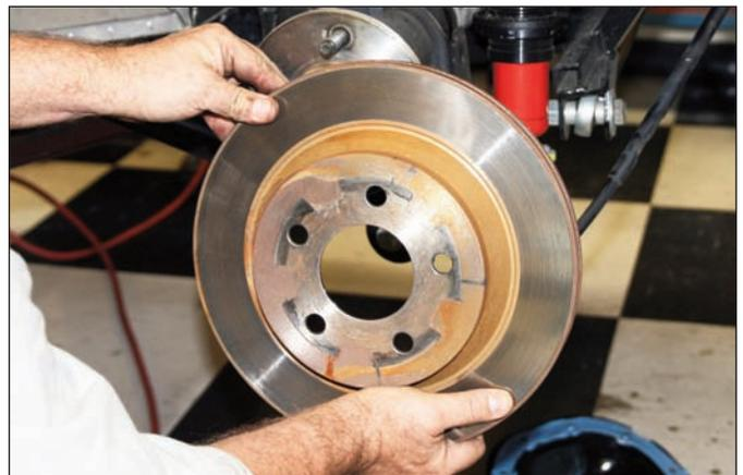
**Sequence 6:** Slide off the rotor from the hub. If it is stuck, it may be necessary to hit it a few times with a rubber mallet to break loose.
