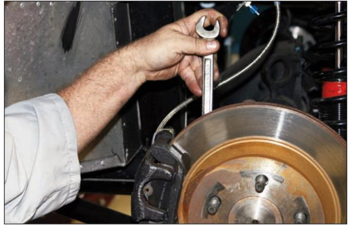
**Sequence 4:** Using a wrench, break loose the caliper mounting bolts from the back side of the rotor.
