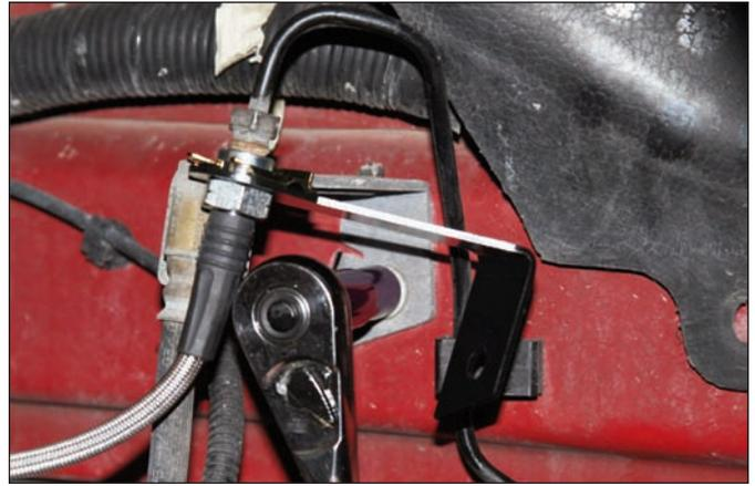
**Sequence 16:** Remove the old mounting bracket from the chassis. Save the mounting bolt.
