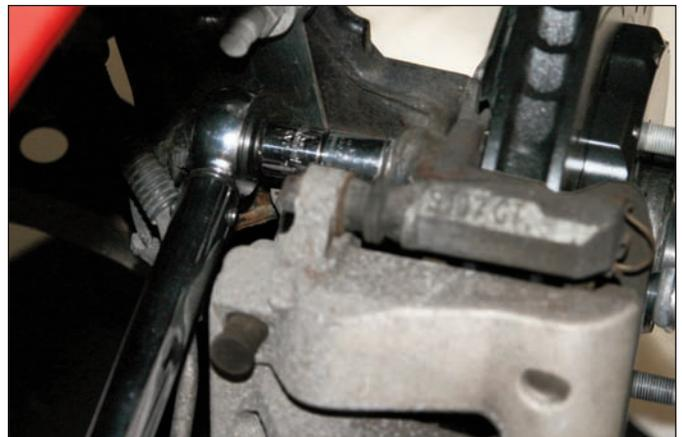
**Sequence 12:** Reinstall the caliper in its original location and torque the mounting bolts to manufacturer's specification.
