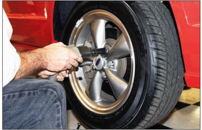
**Sequence 21:** Install the wheel and torque the lug nuts to manufacturer's specification. Rotate the wheel and check for any interference. Bed in the brake pads and rotor in a safe location before general use driving.
