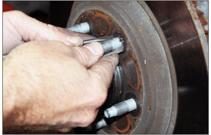
**Sequence 4:** Using a flat head screw driver pry off the rotor retaining washers from around the wheel studs.
