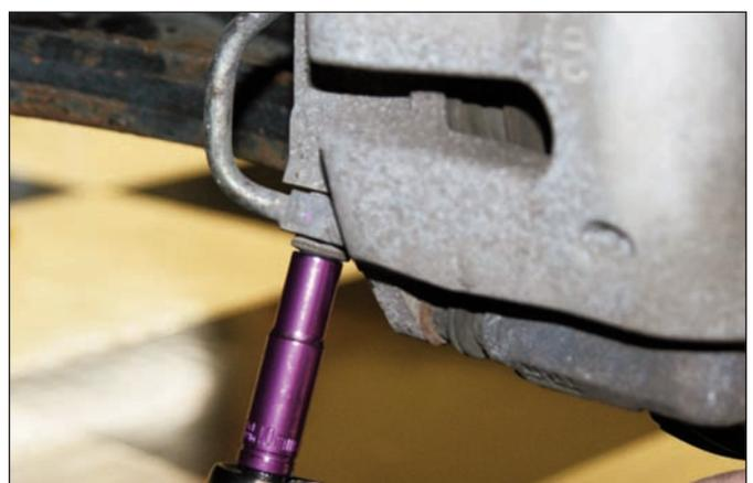
**Sequence 18:** Disconnect the other end of the rubber hose from the caliper. Try to keep fluid leakage to a minimum.
