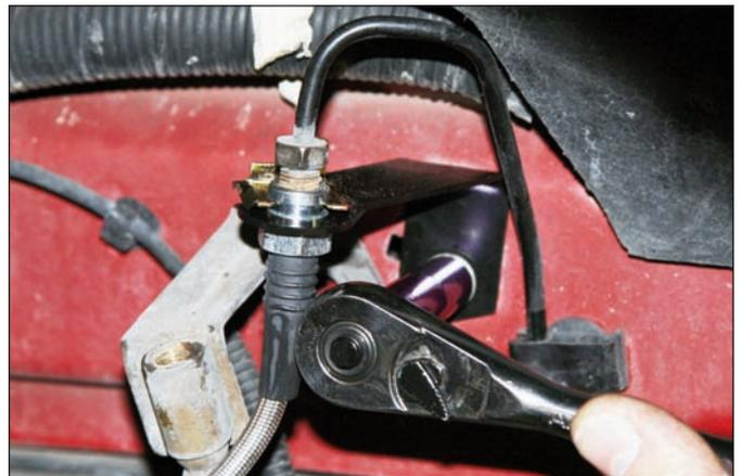
**Sequence 17:** Secure the new mounting bracket to the chassis using the saved OE bolt.
