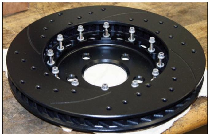
**Sequence 6:** The hat needs to be bolted to the rotor. Orient the rotor over the hat in the configuration shown above. Place one flat washer over each hole on the rotor mounting tabs.
