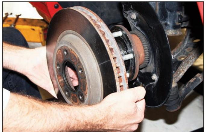
**Sequence 5:** Slide off the rotor from the hub. If it is stuck, it may be necessary to hit it a few times with a rubber mallet to break loose.
