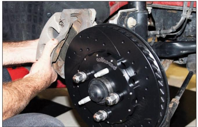
**Sequence 11:** Remove the original brake pads from the caliper and insert new Wilwood brake pads with the friction material facing the rotor.
