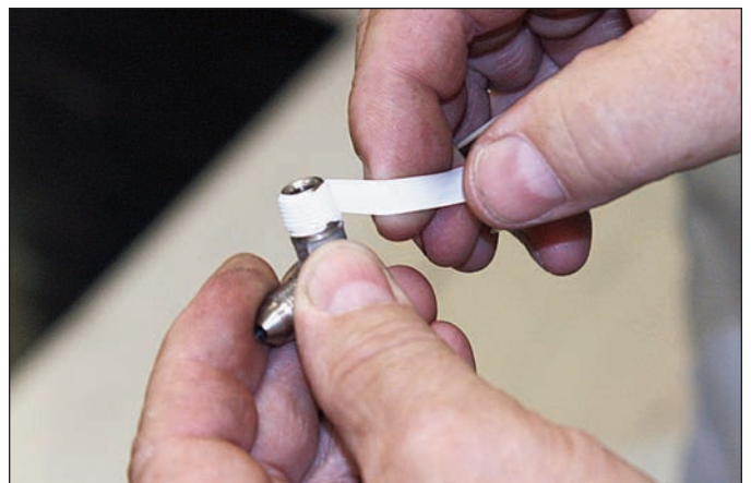
Sequence 18: Remove the protective sticker from the caliper fluid inlet. Wrap the inlet fitting with PTFE thread tape and screw into the caliper in the vertical up position with the fitting angled approximately 45° toward the hard line.
