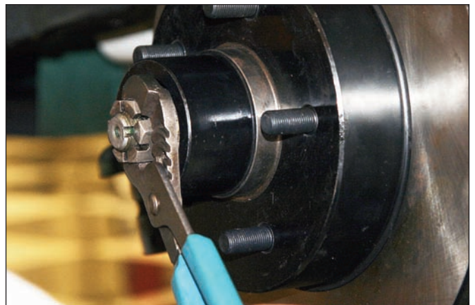
Sequence 17: Install spindle nut. Adjust bearings by tightening the wheel bearing nut to 60 in-lbs. while turning the hub/rotor assembly. Back off the adjusting nut one slot and install a new cotter pin (not supplied). The resulting adjustment should be zero (no pre-load to 0.003 inch end play).
