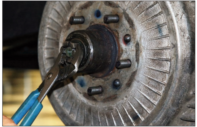
Sequence 4: Unscrew the spindle nut. NOTE: The spindle threads are left hand on the driver's side and right hand on the passenger's side.
