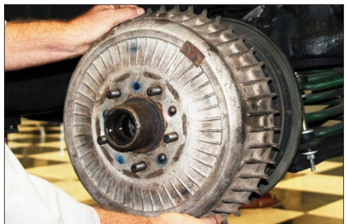
Sequence 5: Lift off the brake drum and set aside.
