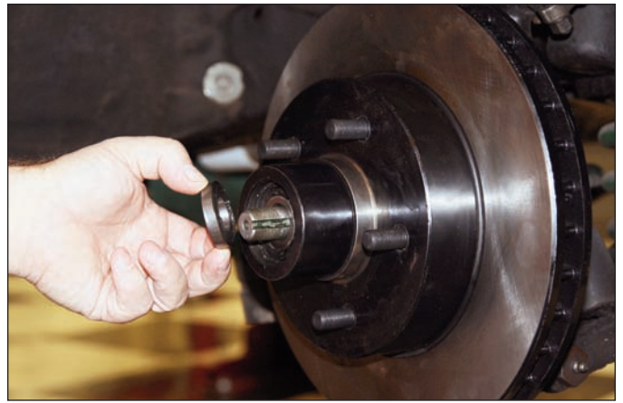
Sequence 16: Install spacer onto the spindle followed by the spindle washer.
