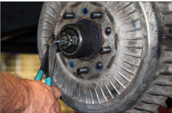
Sequence 3: Straighten out the cotter pin and remove.
