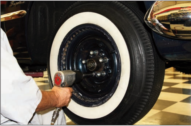
Sequence 1: Raise the front wheels off the ground and support the front suspension according to the vehicle's manufacturer's instructions. Remove the lug nuts, then slide off the wheel.
