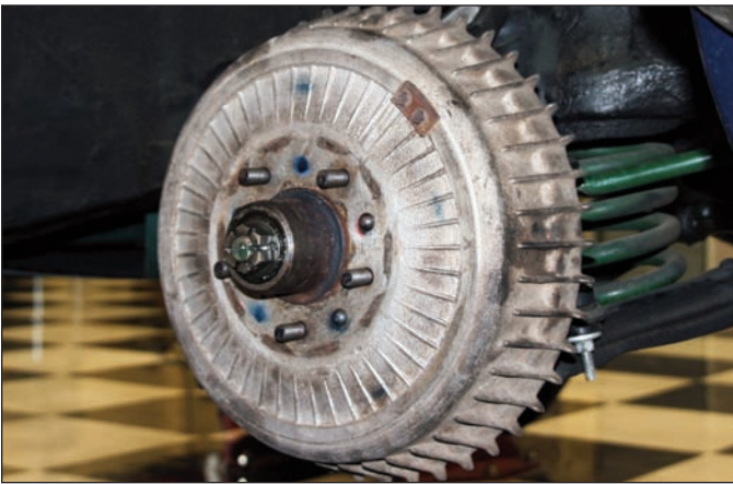
Sequence 2: Remove the dust cap.
