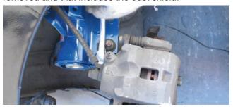
Using a socket wrench, the two bolts fastening the caliper to the hub assembly were disconnected.
