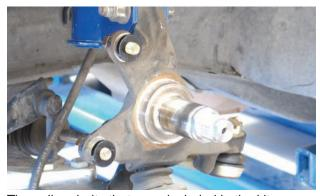
The caliper bolts that were included in the kit were installed in the original spindle assembly along with the sleeves. Notice that this kit also uses a spacer on each bolt along with a 0.016-inch thick washer.
