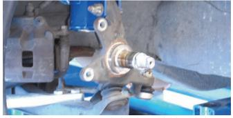
After the hub was removed, the dust shield could be accessed and it can be removed. The Wilwood brakes will be installed without a dust shield.
