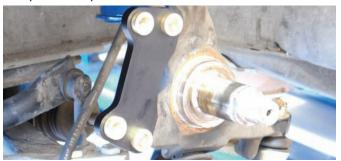
Here is the Wilwood caliper bracket after it was installed. The bracket was bolted on with two 1 ½-inch long 7/16-20 bolts followed by a 0.063-inch thick washer. The bolt goes though a sleeve and on the other side of the spindle there is a small spacer and another 0.016-inch thick washer. Notice the curve on the inside of the bracket to allow clearance for the hub assembly.
