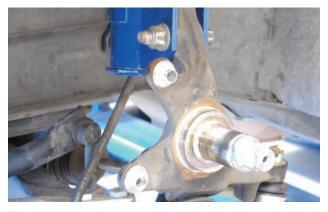
The original caliper mounting holes are large, so they will have to be sleeved down to the size of the Wilwood caliper mounting bolts. The sleeves are included in the kit.
