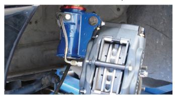
Here you can see the feed line running to the caliper mounting fitting. This line should be very tight to avoid any possible chance of leaking.
