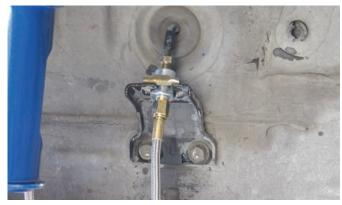
The other end of the stainless steel line was run to the original bracket that was outfitted with an adapter fitting that mates the original steel line to the Wilwood Flexline.
