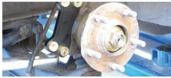
The hub was reinstalled on the spindle and tightened properly. This spindle bolt is a special locknut.
