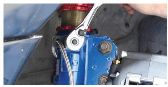
The Wilwood part number 220-9199 stainless steel line was secured to the strut with a small clip as seen here.
