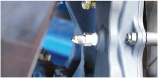
The inlet fitting threads were coated with Teflon tape and then the inlet fitting was screwed into the side of the caliper.
