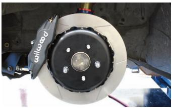
The Wilwood brake system looks great and will improve the stopping power of this 240SX on the street and on the track. At this point the brakes will have to be bled and the brakes will have to be bedded in following the directions on the instruction sheet.
