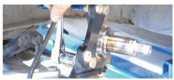
The Wilwood caliper bracket was connected to the spindle assembly and it was tightened in order to check the caliper to rotor centering. The caliper bolts were coated with Loctite and they were tightened to 75 ft-lbs using a foot-pound torque wrench.
