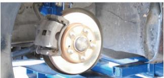
After the wheels were removed you can see the factory disc brake system. This assembly will have to be removed and that includes the dust shield.
