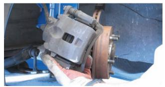
The heavy cast iron brake was removed from the assembly. In order to do that the hose leading to the hard line connection was disconnected. The line was plugged off to keep the line from leaking.
