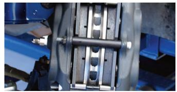
After the pads were in place, the caliper bridge bolt was installed. A close look reveals that the pads are centered perfectly and the radius of the pads matches the radius of the rotors.
