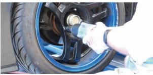
The front of the car was raised with a floor jack followed by the installation of jack stands underneath the chassis. Using an impact gun and the appropriately sized socket, the lug nuts were disconnected and the wheels and tires were removed.
