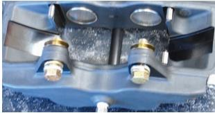
The caliper was bolted to the caliper bracket with two 1  $\frac{1}{2}$ -inch long 7/16-20 bolts. The bolt should be outfitted with a 0.063-inch washer on the outside of the caliper and in this case two 0.016-inch thick shims between the caliper and bracket. The shims are used to center the caliper over the rotor so the total number of shims used may change.
