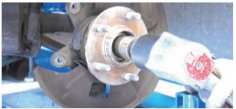
In order to remove the dust shield, the hub assembly will have to be removed from the spindle. Using an impact gun, the large spindle bolt was removed.
