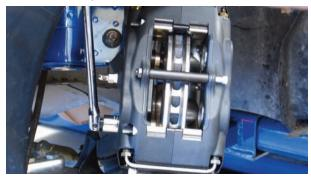
The caliper was centered over the rotor and when it was perfect, the caliper bolts were coated with Loctite 271 and were then tightened to 75 ft-lbs using a foot-pound torque wrench.
