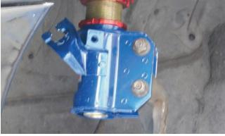
The strut has a built-in hose bracket, but in this installation a different clip will be used to mount the hose.
