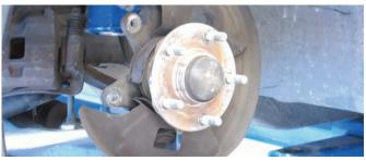
The factory rotor was removed from the assembly and here you can see the dust shield and the caliper mounting ears that will be the mounting location for the Wilwood caliper brackets.
