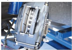
The caliper bridge bolt was removed and the BP-10 Smart Pads were installed.
