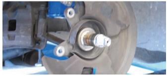
After the hub was removed, the dust shield could be accessed and it can be removed. The Wilwood brakes will be installed without a dust shield.
