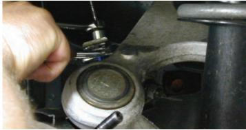
The old hose was removed from the hard line and new the new flex lines were installed.
