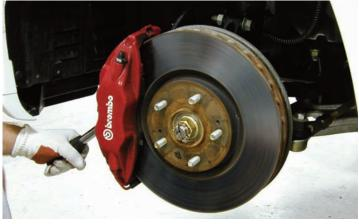
Using a breaker bar and the correct size socket, the two bolts securing the caliper to the bracket were disconnected.
