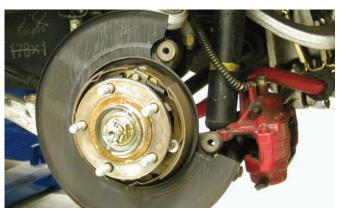
After the caliper was disconnected, the rotor was removed and that shows the original internal parking brake mechanism. Here you can also see the two caliper mounting ears that will be used to mount the Wilwood caliper bracket.
