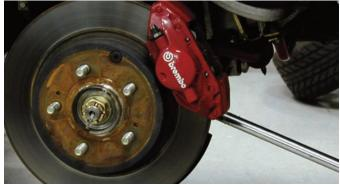
Using a breaker bar and the correct size socket the two bolts securing the original caliper were loosened.
