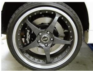
Here is the finished brake system after the large diameter wheels were installed. The large windows certainly gives onlookers a good view of the brakes being used on the car.
