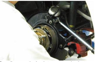
The caliper mounting bracket was secured to the two mounting ears with the bolts and washers supplied. The 35mm bolt was loaded with a 0.095-inch thick lock washer and a 0.020-inch thick shim washer was used between the bracket and the mounting ears. After the caliper to rotor centering was correct, the bolts were coated with Loctite 271 and they were tightened to 35 ft-lbs.
