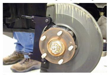
The bolt and 0.063-inch thick washer was placed through the mounting ears and then it was loaded with a 0.033-inch thick and a 0.015-inch thick washer before it was bolted to the bracket. Shims can be used between the bracket and the mounting ears if rotor centering is required.
