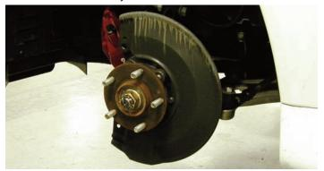
After the rotor was removed you can see the dust shield and the two original caliper mounting ears. The Wilwood caliper bracket will connect to the mounting ears.
