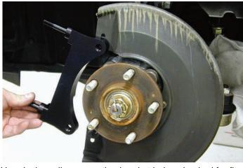
Here is the caliper mounting bracket being checked for fit. The bracket will bolt to the original caliper mounting ears.
