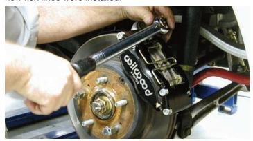
After the caliper was installed and the rotor was centered, the 0.057-inch thick washers were installed and the 3/8-24 self-locking hex head nuts were tightened to 35 ft-lbs.
