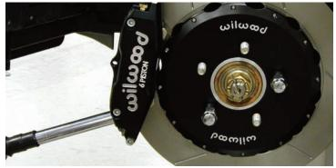
The caliper bracket mounting bolts were coated with Loctite 271 and then they were tightened to 100 ft-lbs using a footpound torque wrench.
