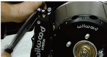
After the two self-locking nuts were snug, they were tightened to 35 ft-lbs using a foot-pound torque wrench.
