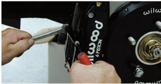
The bridge bolt was installed in the caliper and then it was tightened with an open-end wrench and an Allen T-handle.
