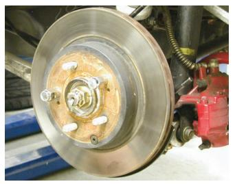
Since this is the prototype car for this installation kit, the original style rear rotors are being used while the aluminum hat rotors are being developed. Here the rotor is connected to the hub with a pair of lug nuts.
