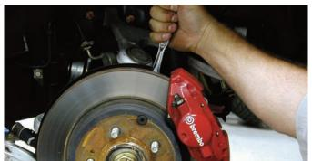
After the breaker bar loosened the bolts, they were removed with a smaller socket wrench as seen here.
