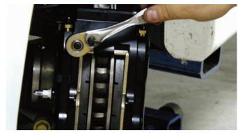
Using a small socket wrench, the two 3/8-24 self-locking hex head nuts were tightened. A 0.057-inch thick washer was used under each nut.
