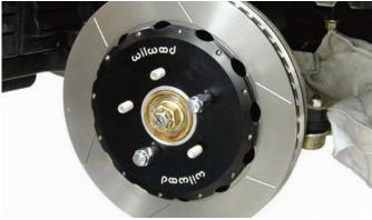
Two lug bolts were used to secure the rotor to the hub assembly so the rotor to caliper centering could be determined.
