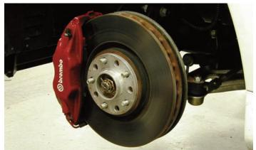
Here are the front brakes that come standard on the car. The Brembo brakes are better than what you will find on other Mitsubishi products but they are heavy and the car's stopping power and handling can be improved.
