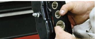
The caliper inlet fitting was wrapped with Teflon tape and then it was screwed into the side of the caliper as seen here. This also gives you a chance to see the six pistons in the caliper. It would be good to note that sixpiston calipers are marked right and left.
