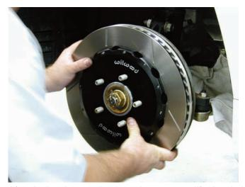
After the bracket was in place, the rotor was lifted and placed on the hub assembly as seen here. The aluminum hat was connected to the rotor using the bolts and washers in the kit. The bolts were coated with Loctite 271 and then they were tightened to 85 in-lbs in an alternating sequence using an inch-pound torque wrench.
