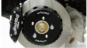
Here is the finished brake assembly ready for the brake hose installation. The brakes will work great and they also look nice.
