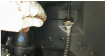
Using a line wrench, the hard line was disconnected from the flexible line. This bracket will also be used to mount the Wilwood brake hose.
