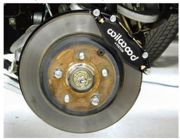
The rear brakes are finished and now the car is ready for brake bleeding and pad bedding. This system works terrific and the owner said the car performs great on the street and even better on the track.
