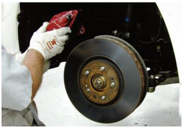
After the caliper bolts were disconnected the caliper was removed from the assembly.
