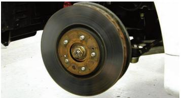
The next step was removing the rotor from the assembly. It may take a little persuasion to get the rotor to separate from the hub assembly.
