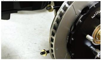
The caliper mounting bracket studs were loaded with a 0.47-inch long spacer and a 0.035-inch thick shim washer before the caliper was installed.
