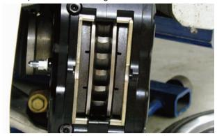
Here is the caliper after it was mounted and as you can see the rotor is centered perfectly. Notice that the radius of the brake pads matches the radius of the rotor assembly.
