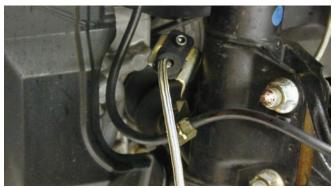
The original mounting bracket for the hose was reused to keep the line away from moving parts.
