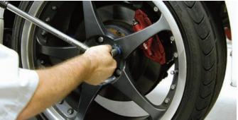
The front of the car was lowered after the jack stands were removed. The rear of the car was elevated and jack stands were carefully placed under the car. Now the rear wheels and tires were removed as seen here.
