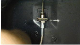
The cap was removed from the adapter fitting and then the braided steel line was connected.
