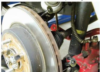
A close look reveals a pair of 0.035-inch thick washers were installed, one on each stud before the caliper was installed.
