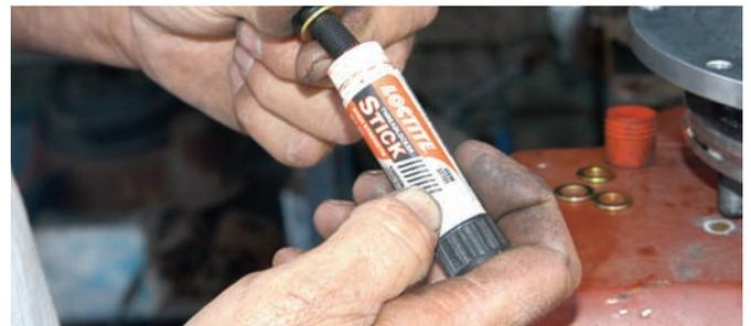
The hub has to be connected to an aluminum spacer ring. This must remain tight so the high strength Allen head button bolts were coated with Loktite to keep the bolts from backing out.
