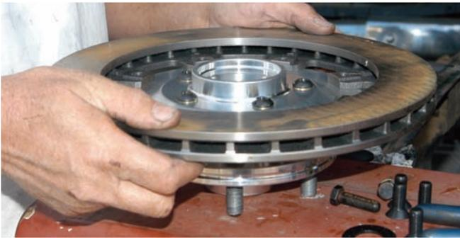
Now the steel rotor can be connected to the aluminum hub assembly. Take a close look at how the mounting tabs for the rotors face forward.
