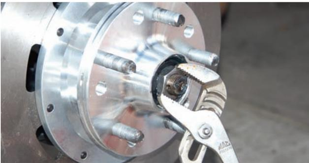
The spindle nut was installed with channel lock pliers and it was tightened to the point of being snug, but not too tight. If the nut is cranked down tight, the bearings will wear out prematurely.
