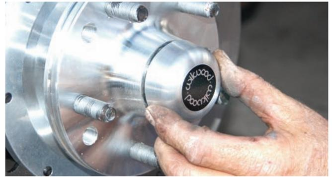
Installing the screw-on grease cap finished the front spindle assembly. The cap is easy to install and it looks nice.
