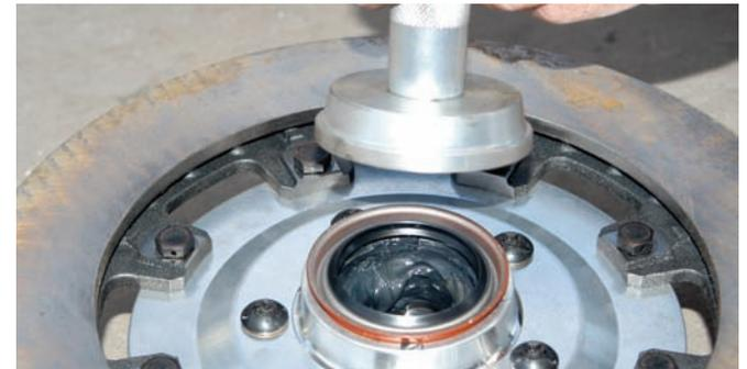
The seal was secured in the hub with this seal installation tool. A few taps with the hammer and the seal is secured in the hub.
