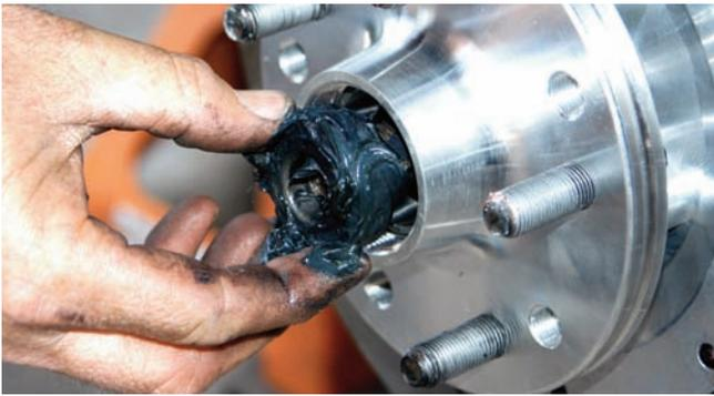
The small front bearing was also packed with grease and then it was installed over the spindle and into the front bearing race.
