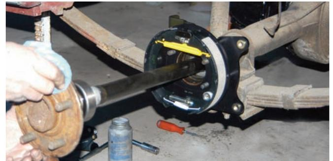
The axle was loaded into the axle assembly making sure that the splines at the end are lined up properly. You can feel the axle slip inward when the splines line up.
