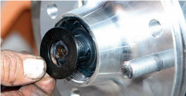
The large washer that was supplied in the kit was installed next. This washer will keep the front bearing securely in the rotor.
