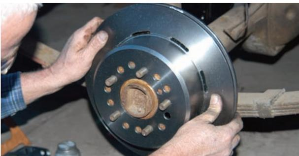
The rear rotor was installed on the axle flange. Notice that the rotor has several holes drilled into it making it a universal part. The bolts that match the Ford lug pattern were selected.
