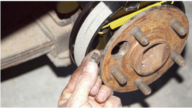
A horseshoe shaped bracket secures the parking brake unit and caliper bracket to the housing and it is secured with four locknuts. Here one of the locknuts was being installed.
