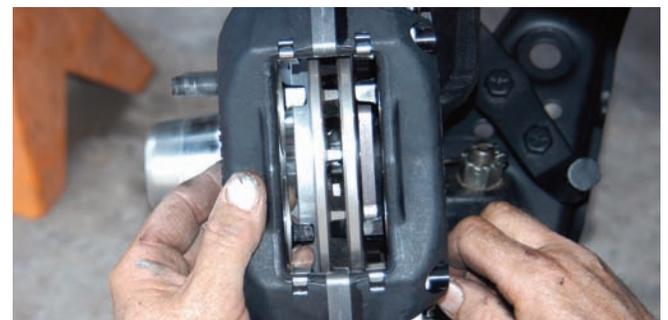
The rotor has to be centered inside of the caliper. Shims are included in the kit to make this possible. Here the rotor is centered and ready to go.
