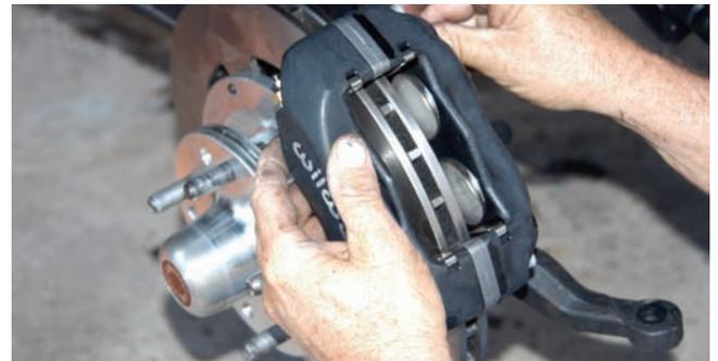
The large caliper was installed next and it was secured with the two mounting bolts included in the kit. It would be a good idea to coat the installation bolts with Loctite so they stay secure.
