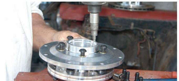
The Allen head button bolts were tightened with an impact gun. If you try to do this with wrenches the bolts will not be tight enough. After the bolts are snug they should be tightened to 180 in-lbs using an inch-pound torque wrench.
