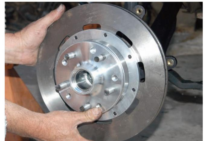
The rotor assembly was lifted and it was installed on the spindle. Here is a good look at the rotor assembly after it was loaded on the spindle.
