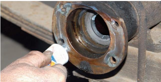
The flange was coated with silicon to prevent oil leaks. The four special head flange bolts were installed.
