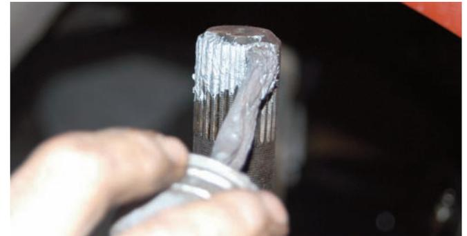
The splined end of the axle was coated with anti seize lubricant to make it easier to install and remove later if necessary.
