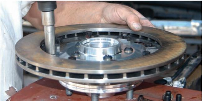
The rotor bolts were coated with Loctite and then they were installed with an impact gun. The bolts should be tightened to 22 ft-lbs using a foot-pound torque wrench.
