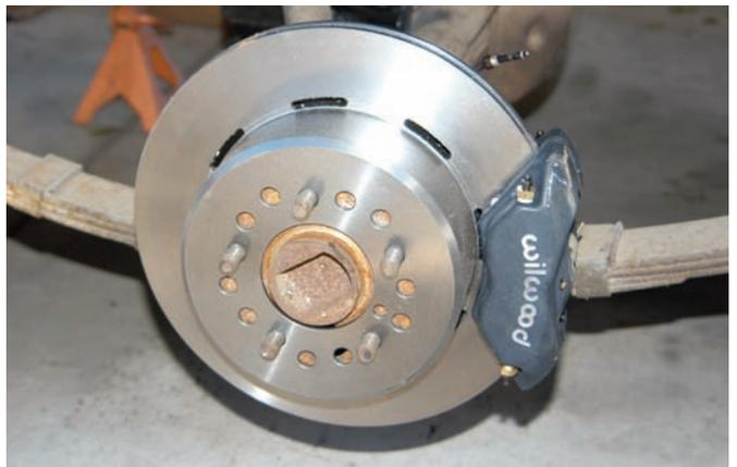
Here is the rear brake system after it was installed. The large caliper and rotor provide excellent stopping power and the internal emergency brake works great. This Fairlane convertible finally has brakes that can bring this 390ci powered car to a quick stop in any situation.
