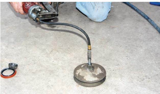
The upper section was installed and then the fitting on the top was connected to a grease gun. The gun pumped the grease into the small tool and it was forced to go through the bearing.
