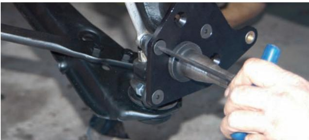
Using an Allen wrench and an open-end 9/16 wrench, the brackets were secured to the spindles. Notice there are two additional holes in the bracket so it can also be used on another Ford spindle style.
