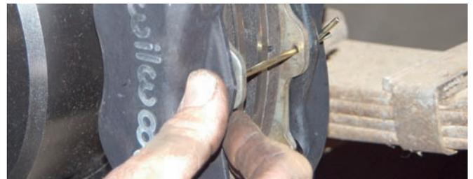
The pads were secured with a long cotter key. The end of the key should be bent over enough to keep it in place but not too much because it will have to be straightened when the car needs new pads.
