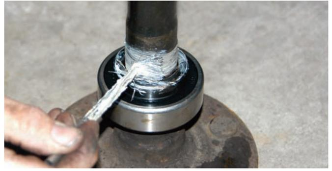
Since the axle had to be removed to install the brakes, the installer thought changing the axle bearing would be a good idea. The area that will ride in the axle seal was coated with white grease.
