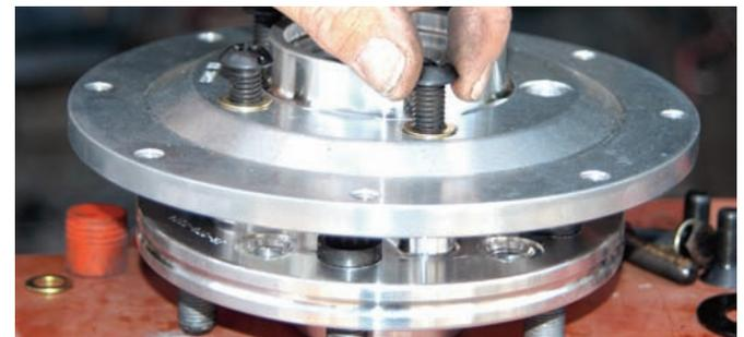
Take a close look at the spacer ring because the dished portion has to face forward. It can be bolted on the other way but the rotor will not line up with the caliper.
