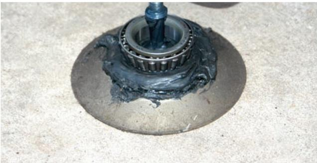
After the rotors are assembled they can be installed on the spindles. First the bearings have to be packed with grease. This can be done by hand or with a packing tool so we will show you how it works. The bearing was installed in the lower section.
