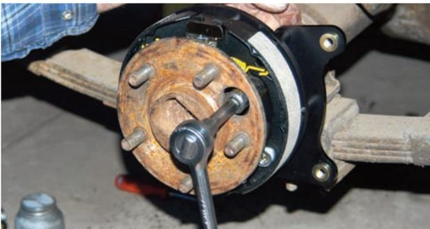
The axle flange features an axle bolt access hole. Here the bolt is being secured with a socket wrench. This photo also gives you a good look at the caliper bracket.
