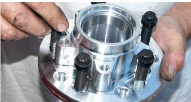
The aluminum hubs are drilled with two bolt patterns, Ford-Chrysler 5 x 4.5 and Chevy-Pontiac-Olds that is 5 x 4.75. The Ford pattern was selected for this application.
