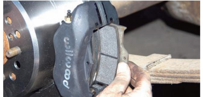
The brake pads were installed in the calipers from the top. These are large calipers so they should work great on this lightweight Fairlane. The calipers were being equipped with BP-10 smart pads.
