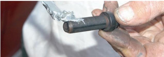
The lug bolts do not come installed in the hub, so the installer has to install them using the correct bolt pattern for the car. Since the lug bolts are steel and the hubs are aluminum it is a good idea to coat the lugs with anti seize before they are installed.
