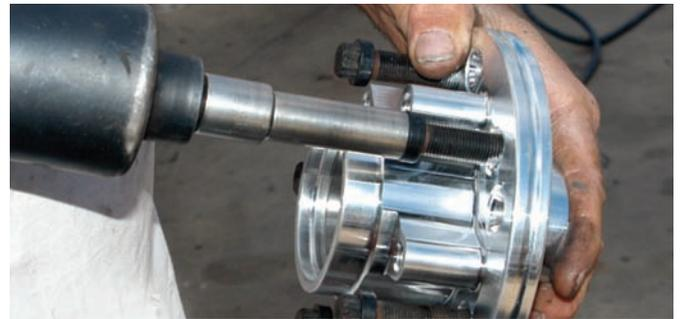
The Studs were installed with an impact gun because it does a good job of tightening the lugs. They should be tightened to 77 ft-lbs using a foot-pound torque wrench.
