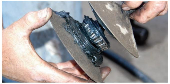
The top section of the tool was removed and you can see that the bearing was packed with grease. This tool is great, but if you don't have one the packing can be done by hand.
