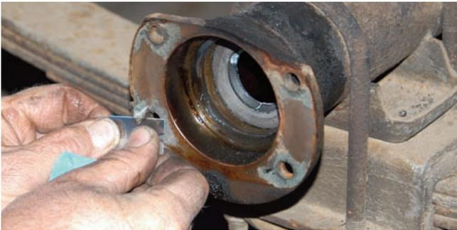
Now the rear brakes can be installed. Cleaning the old gasket off of the differential flange assembly with a razor blade started the procedure.
