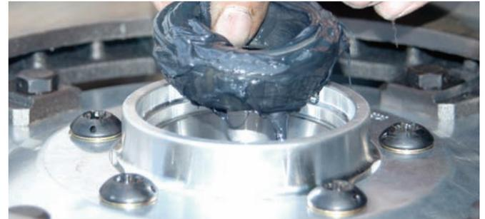
The coated bearing was installed in the aluminum rotor and hub assembly. The hub is delivered in the kit with the correct races installed.
