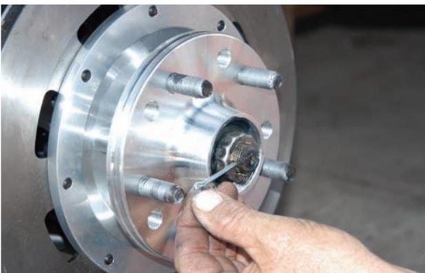
After the nut was tight, a castle nut cover was installed along with a cotter key to keep it from backing out. This is a very important safety procedure so make sure the cotter key is used.
