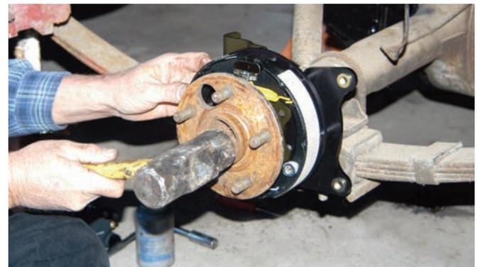
The splines were lined up in the differential, but some persuasion was needed to get the axle bearing to bottom out in the housing.
