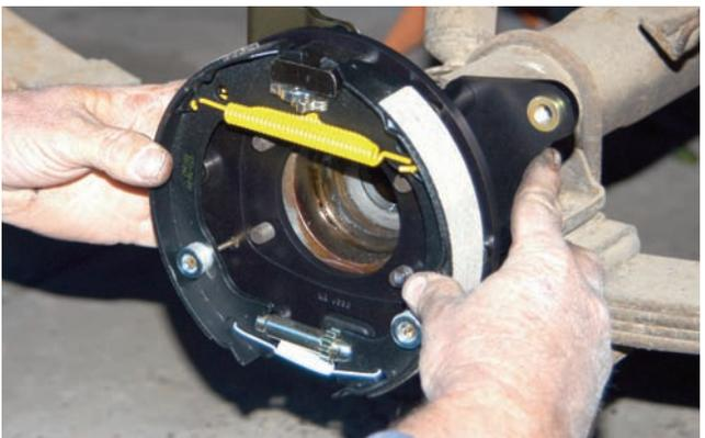
The small emergency brake assembly was installed over the four flange bolts. The assembly is actually a miniature drum brake and it also features a bracket for the caliper that will be installed later.
