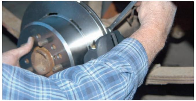
The mounting bolts were coated with Loctite and then they were screwed into the mounting bracket. Here the bolts are being tightened with a long 9/16-inch wrench.
