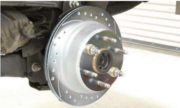
The rotor was connected to the axle assembly with two opposing lug nuts so the rotor to caliper centering could be done.
