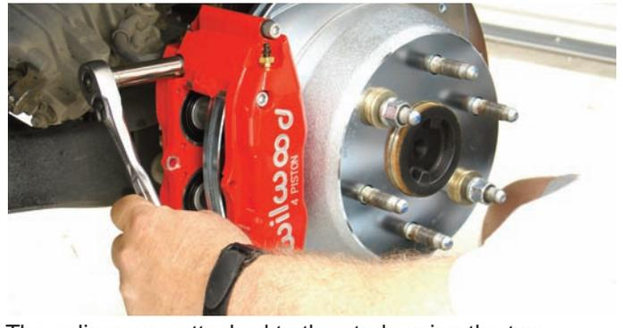
The caliper was attached to the studs using the two 0.057-inch thick washers and two self-locking hex head nuts. The rotor to centering should be checked and adjusted if necessary at this point. Shims between the caliper bracket and the original mounting ears can be used if necessary.
