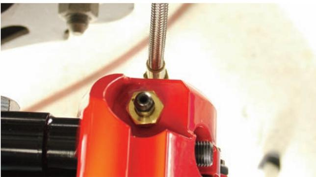
The hose connection was made from the caliper to the hard line. At this point the old caliper can be removed. The brake system will require bleeding and the pads will have to be bedded in.
