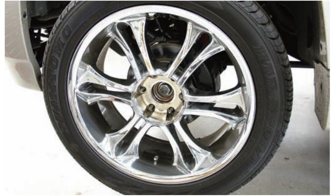
The Denali was raised up on a floor jack and then jack stands were installed underneath for safety. The hub-caps were removed and the lug nuts were disconnected with an impact gun and the correct size socket. After the lug nuts were disconnected, the large wheels and tires were removed.
