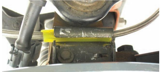
The other bracket was connected to the spindle assembly. The brackets were removed, spread apart enough to get the new hose and plastic protector inside and then the bracket was squeezed back together to secure the hose.
