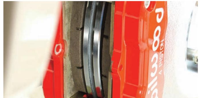
The brake pads are centered over the rotor and the radius of the brake pads match the radius of the rotors. At this point everything is looking good.
