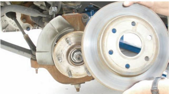
The rotor was lifted off of the hub assembly and was removed from the car.
