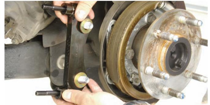
The caliper will be mounted to the original caliper mounting ears using a pair of M-14-2.00 x 40 mm bolts loaded with M14 I.D. x 21mm O.D. lock washers. After the bolts pass through the bracket they should be loaded with a 0.029-inch thick washer before the connection is made.
