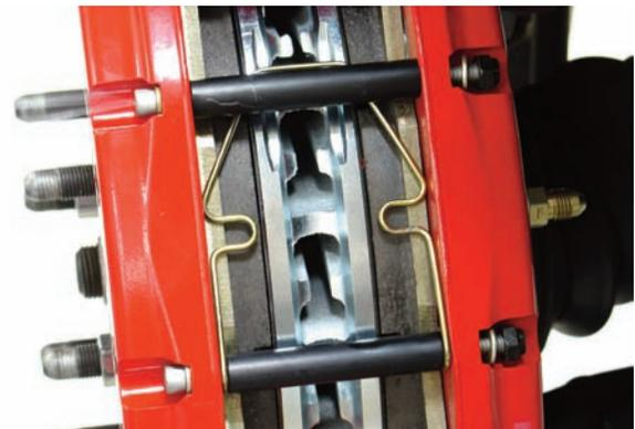
The two bridge bolts were installed along with the wire spring clip. The spring clip can be tricky to get in place.
