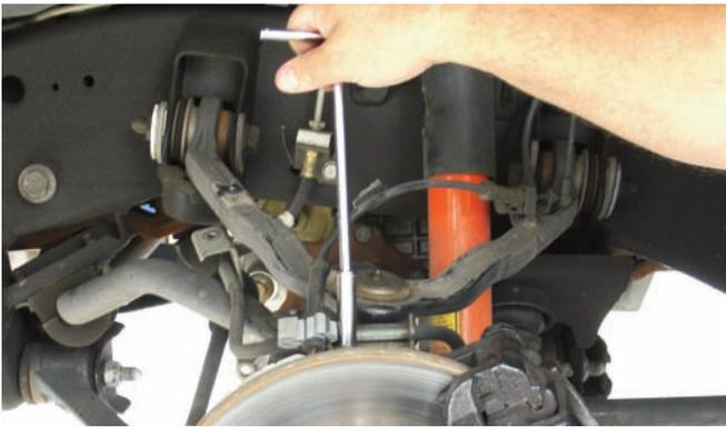
There is another hose bracket located on the top of the spindle. Using a T-handle and a small socket, the retaining bolt was disconnected from the spindle. This bracket will also be reused later.
