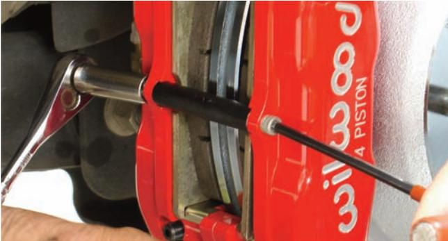
The caliper center bridge pad retainer bolt was re-installed and it was tightened with a small socket wrench and a T-handle.
