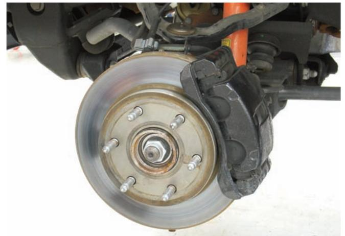
The Denali was raised up on a floor jack and then jack stands were installed underneath for safety. The hub-caps were removed and the lug nuts were disconnected with an impact gun and the correct size socket. After the lug nuts were disconnected, the large wheels and tires were removed.
