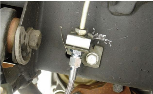
Using an adapter, the stainless steel braided line was hooked to the hard line and both were tightened to avoid leaks. The original clip retainer was reinstalled.
