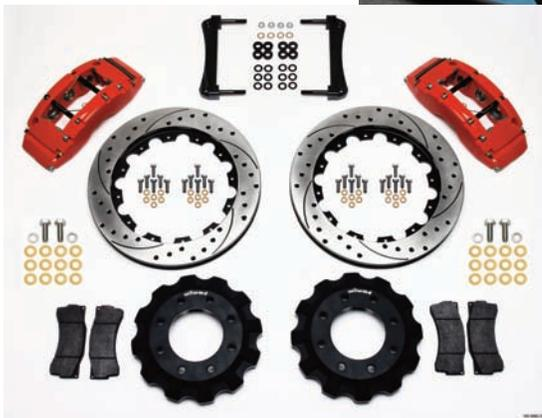
A big vehicle such as this Denali requires large brakes, so a Wilwood part number 140-8992 front disc brake kit was ordered. The kit features huge 16-inch vented and slotted rotors with aluminum hats, TC 6R six-piston calipers, caliper brackets, BP-10 Smart Pads, and all of the hardware required to complete the installation.
