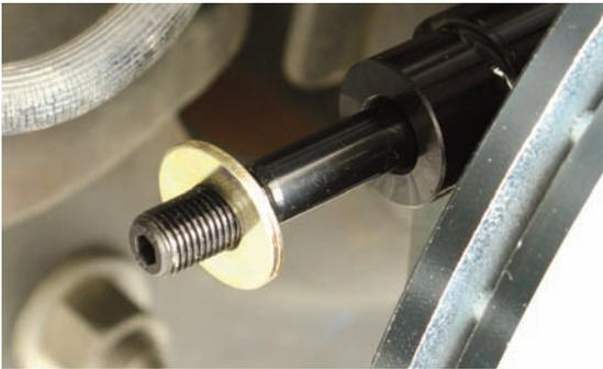
Before the caliper was installed, the caliper bracket studs were loaded with a 0.035-inch thick washer.
