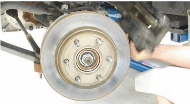
The caliper was lifted off of the rotor and was set to the side for now. It will be completely removed after the rubber line is disconnected from the steel line.
