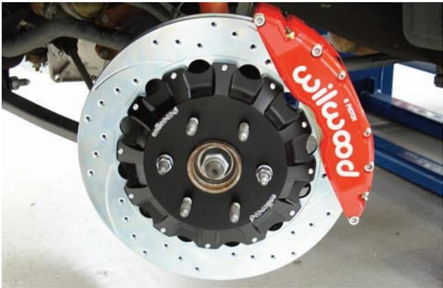
At this point the caliper and rotor are finished, but the brake lines still have to be hooked up. Looking at this system it is obvious that it will be far superior to the original brake system.
