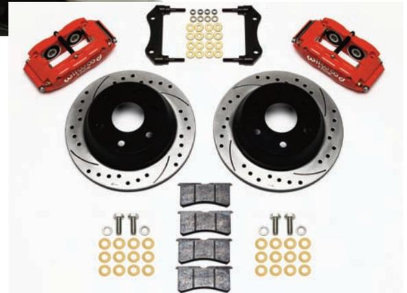
The Denali has an internal parking brake system so a Wilwood part number 140-8993 rear disc brake kit was ordered. The kit features 12.75-inch diameter drilled and slotted rotors with an internal parking brake drum, Superlite 4R calipers, caliper brackets, BP-10 Smart Pads and all of the hardware required to complete the installation.
