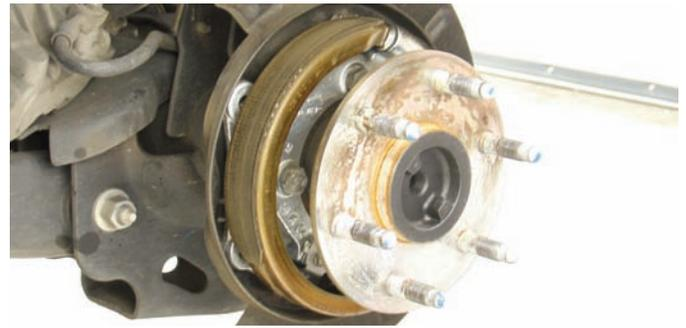
Here is a close look at the internal parking brake assembly. This is a useful assembly so it will be retained, which means the original parking brake cables remain intact.
