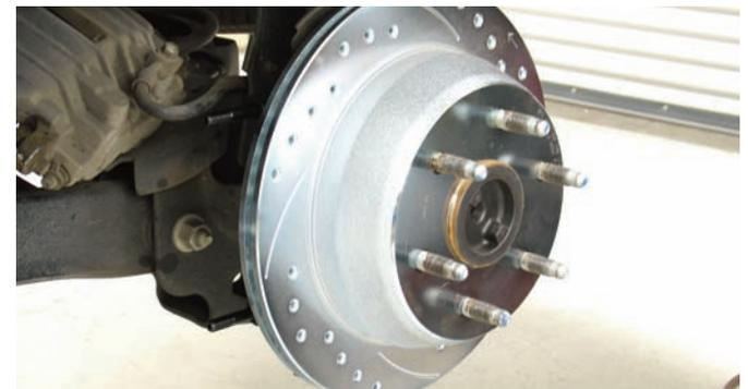
The Wilwood drilled and slotted rotor was installed on the axle flange and was pushed back to mount it on the centering ring. If you look close you can see the caliper bracket mounting studs in the background. This rotor has an internal drum assembly for the parking brake assembly.
