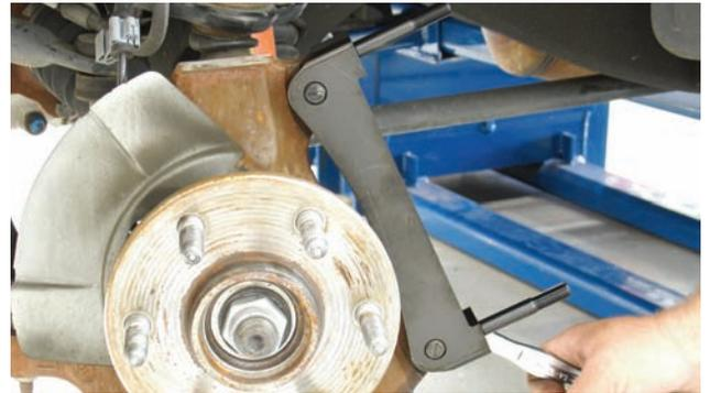
Here is the caliper mounting bracket after it was bolted to the original caliper mounting ears. Shims can be added between the bracket and mounting ears to center the caliper over the rotor.
