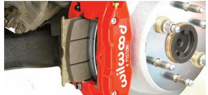
After the caliper was centered, the BP-10 brake pads were installed. The pads are designed for street performance use.
