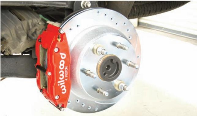
Here is the finished brake assembly featuring the red Superlite four-piston caliper and the drilled and slotted rotor.
