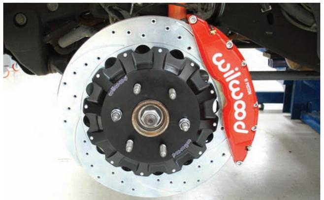
Here is the front brake system complete and ready to go. The brake system features the huge red TC 6R caliper and the 16-inch drilled and slotted rotor. The next step is installing the rear brakes.
