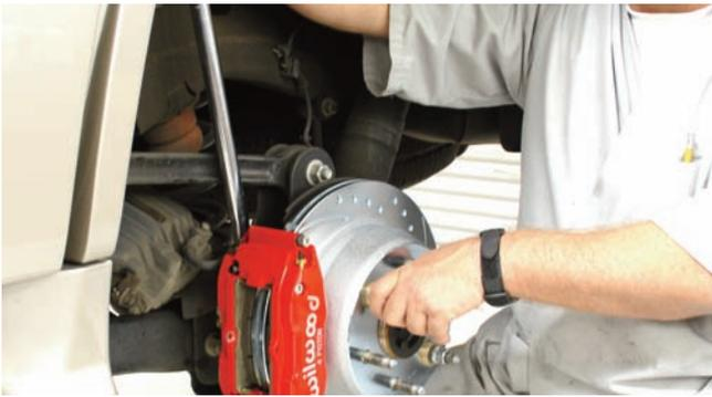
Now the caliper mounting bracket bolts were tightened to 90 ft-lbs using a foot-pound torque wrench.
