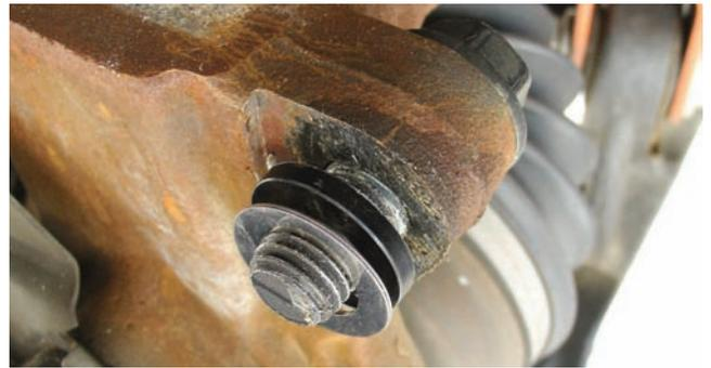
A M14-2.00 bolt outfitted with a M14 lock washer was placed through the hole in original caliper mounting ear and it was loaded with a 0.029-inch thick washer and a thin shim washer in preparation for mounting the caliper.
