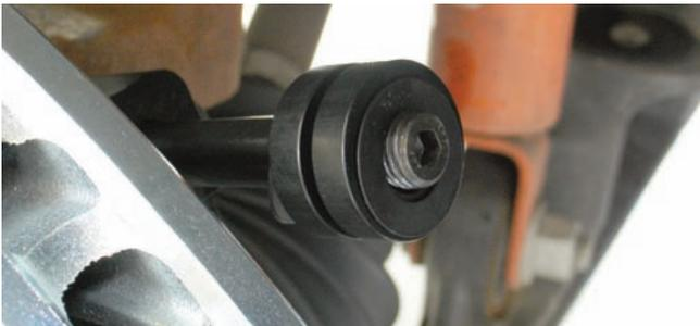
Before the caliper was mounted to the bracket assembly the studs were loaded with two spacers and a shim washer as seen here.
