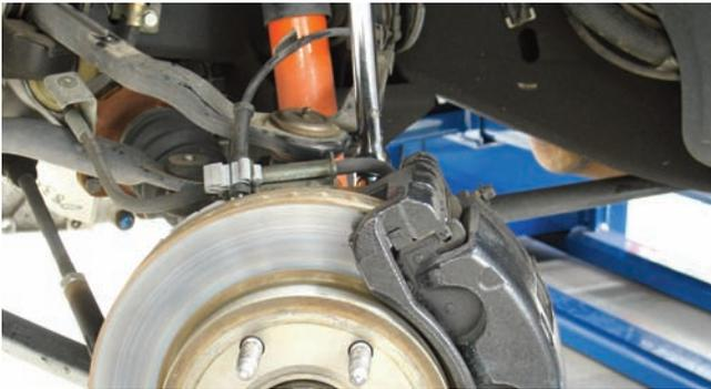
Using a ratchet wrench and the correct size socket, the Caliper bolts were removed from the original bracket assembly. A breaker bar may be necessary to break the bolts loose.
