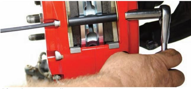
After the spring clip was properly mounted, the two bridge bolts can be tightened using a small socket wrench and an Allen T-handle.
