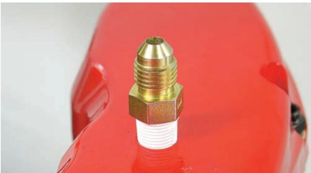
The caliper inlet fitting threads were wrapped with Teflon tape and then the fitting was screwed into the caliper body.
