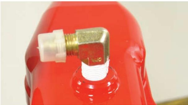
The caliper inlet fitting threads were wrapped with Teflon tape and then the fittings were screwed into the calipers.
