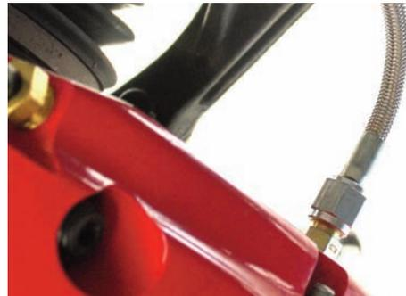
Here is the stainless steel line running to the caliper inlet fitting. It is important to make sure all of the connections are tight.
