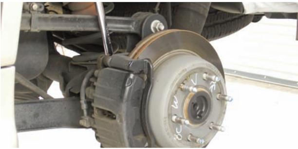
Using a breaker bar and the correct size socket, the caliper bolts were removed.
