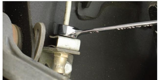
The hard brake line was removed from the rubber hose using a line wrench. The line was loosened but it wasn't removed yet.
