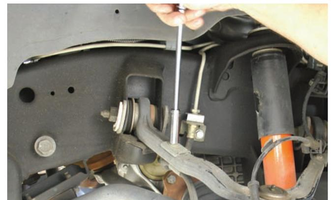
Before the rotor could be removed, the brake line brackets had to be disconnected. Here one of the small brackets was disconnected from the A-arm assembly. It is important to keep the brackets because they will be reused later.
