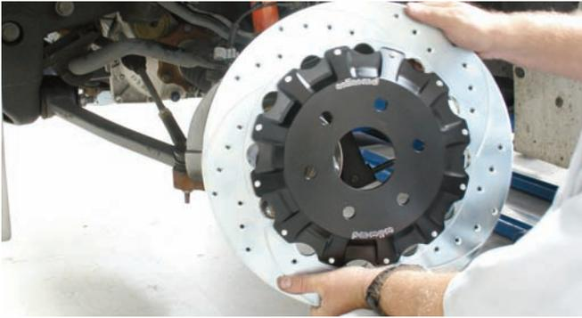
The aluminum hat assembly was bolted to the rotor using the bolts and washers in the kit. The small hub bolts were coated with Loctite 271 before the connection was made and then the bolts were tightened in an alternating pattern to 144 in-lbs using an inch-pound torque wrench. The bolts that were just installed were safety wired together.
