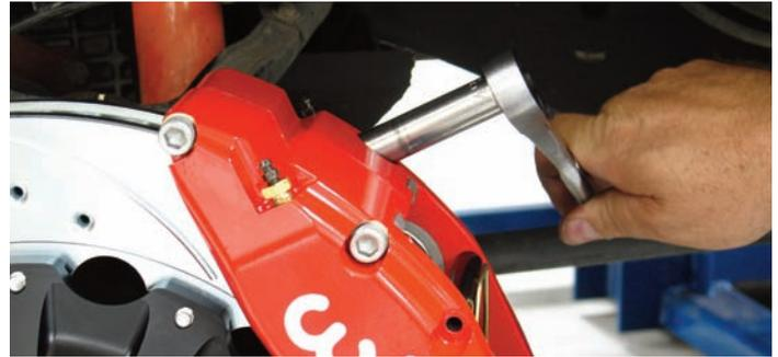
The caliper was placed on the bracket studs and then the washers were installed followed by the locknut. Here the nuts are being tightened in preparation for checking the caliper to rotor centering.
