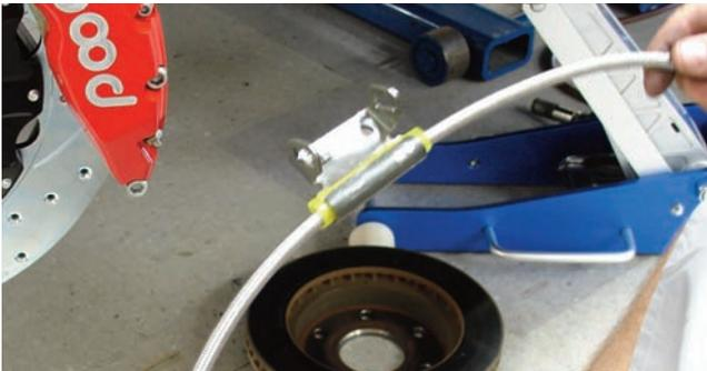
The hose brackets that were previously removed were reinstalled on the new Wilwood part number 220-8998 stainless steel braided line.
