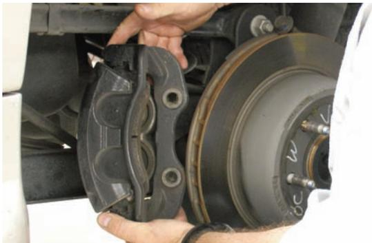
After the bolts were disconnected, the caliper could be removed from the bracket. For now the caliper was just moved out of the way while the new brakes were installed.
