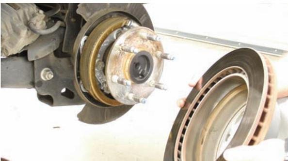
The heavy rotor was lifted off of the axle studs. You can see the original caliper in the background. It will be removed when the new lines are being installed.
