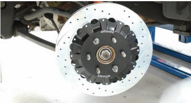
The assembled rotor was mounted on the hub assembly and then it was secured with two lug nuts.
