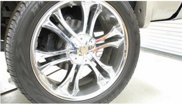
The front of the car was placed back on the ground and the rear was lifted and jack stands were placed underneath for safety. The hubcaps were removed and then the lug nuts were disconnected. After the lug nuts were disconnected the tires and wheels were removed.
