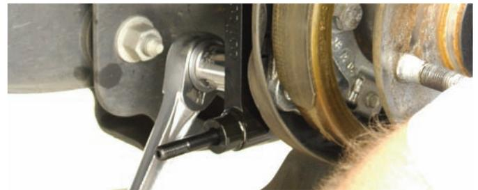
The bolts were installed finger tight and then they were tightened with a socket wrench to check the caliper to rotor centering.
