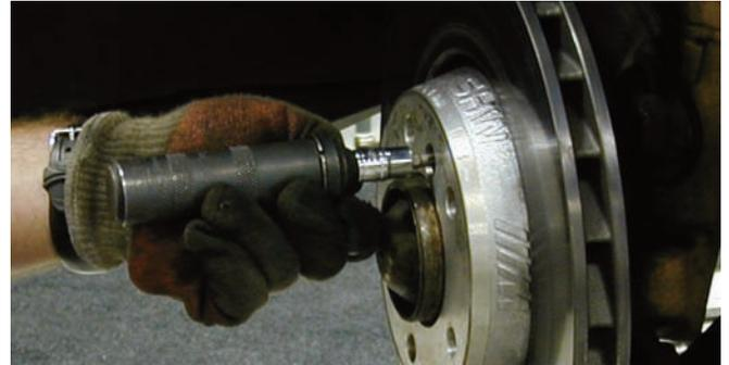
Using an impact screwdriver, the screws that secure the rotor to the hub assembly were disconnected.
