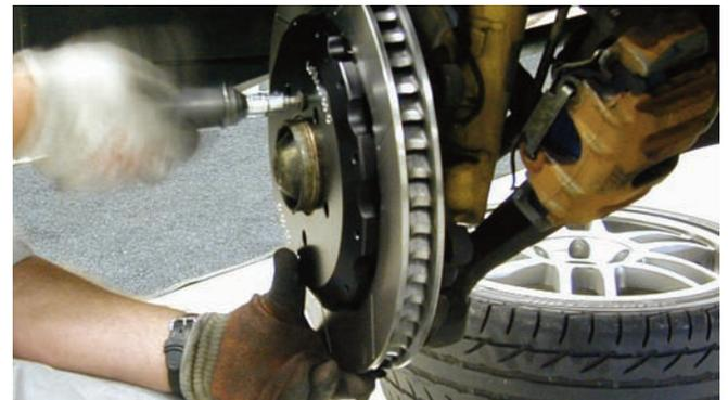
The rotor was connected to the hub assembly using the bolts and washers in the kit. The bolts were coated with Loctite 271 and then they were tightened in an alternating sequence to 85 in-lbs. After the rotor was assembled it was placed on the hub mounting flange and it was connected with the original screws.
