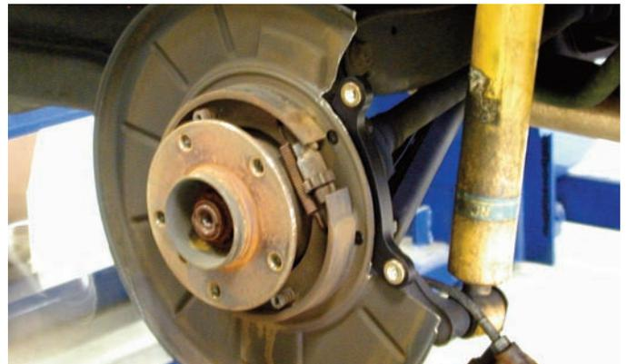
Here is the dust shield after the material was removed. This should allow enough clearance for the new caliper.
