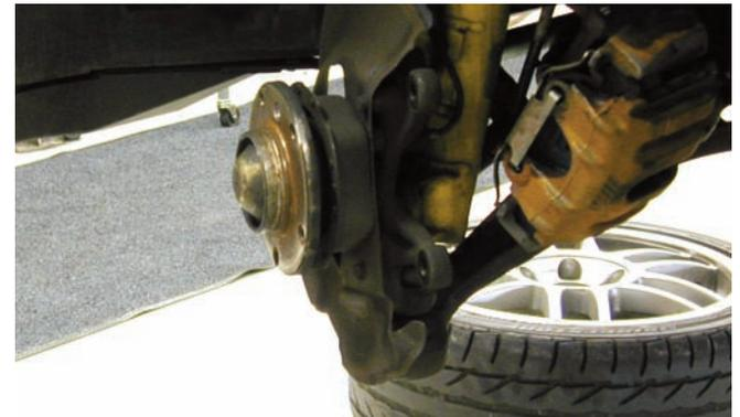
After the rotor was removed, you can see the mounting ears that the caliper bracket will bolt onto.
