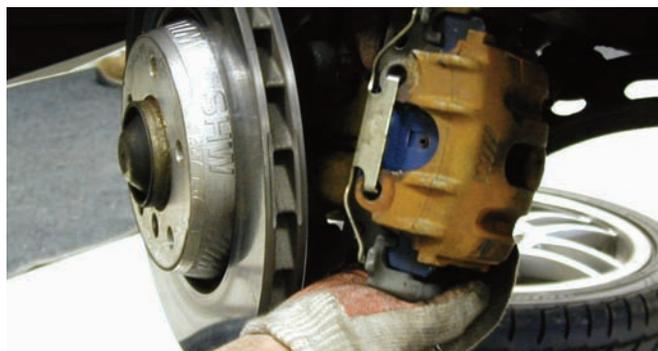
The two bolts that secure the original caliper to the mounting ears were disconnected. After they were removed, the caliper could be lifted off of the rotor.
