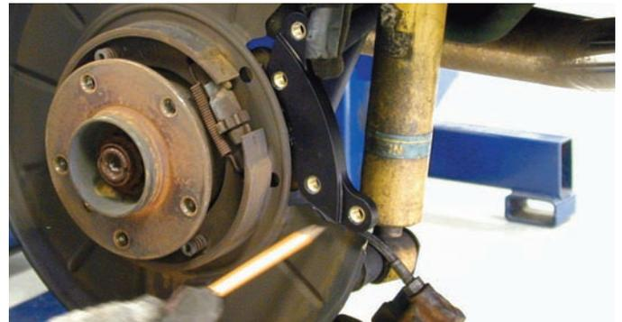
The caliper bracket was connected to the mounting ears to determine where the dust shield will have to be cut to allow the use of a larger rear caliper.
