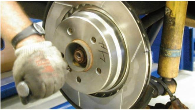
The rotor was placed on the hub assembly and then the original screw was used to secure it. Some parking brake shoe adjustments may be needed to get the shoes close to the hub assembly.
