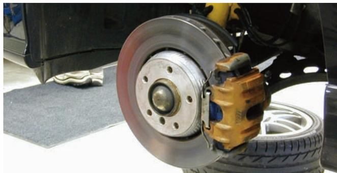
After the wheels and tires were removed, you can see the original disc brake setup. The original calipers are connected to the hub's mounting flange.
