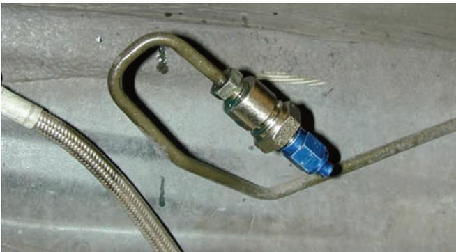
The steel line was moved away from the mounting bracket and an adapter fitting was connected. The blue fitting is just a cap to keep the fluid from leaking out.
