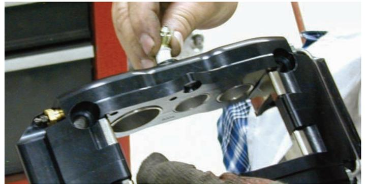
The fluid inlet fitting threads were wrapped with Teflon tape and then the fitting was screwed into the side of the caliper.
