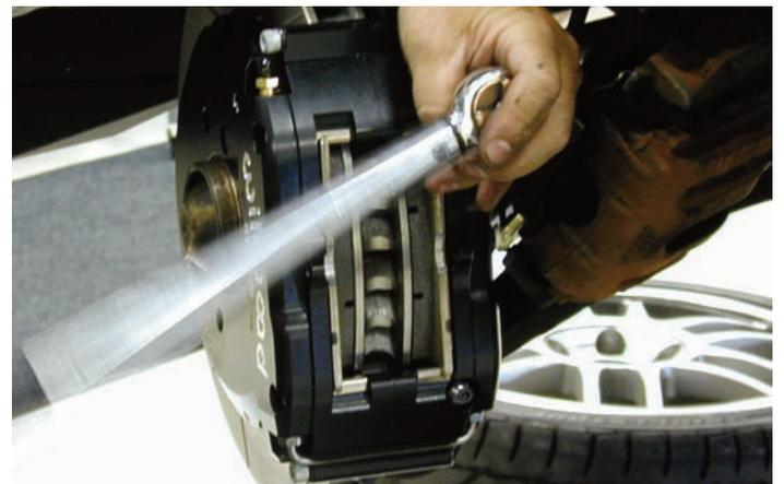
The mounting washers and locknuts were connected to the studs and then the nuts were tightened to 35 ft-lbs using a foot-pound torque wrench.
