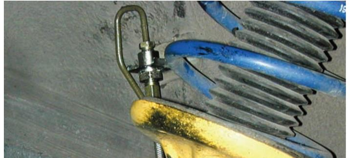
The steel line and adapter fitting were reinstalled in the frame bracket and the Wilwood line was connected. The original brake clip can be used to hold the line in place.
