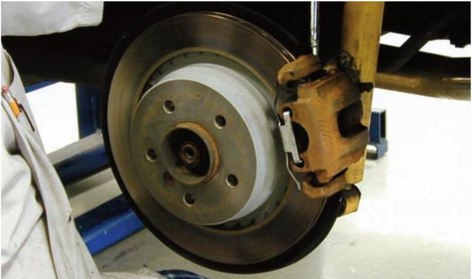
The two bolts that secure the caliper to the bracket were removed with a large breaker bar. After the bolts were disconnected the caliper was removed from the rotor.
