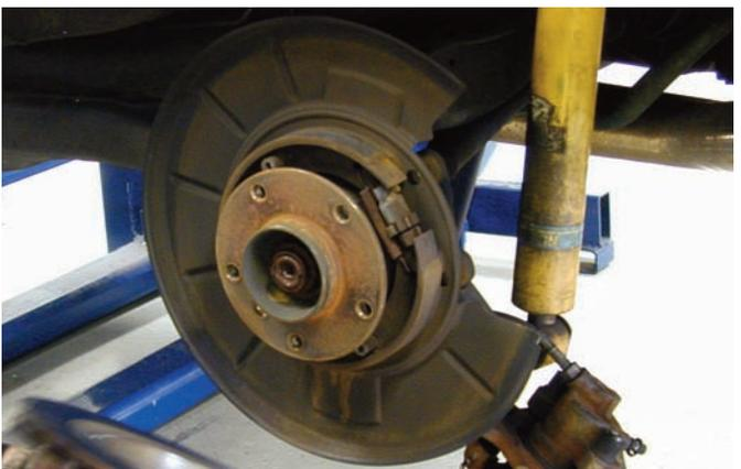
After the rotor was removed, you can see the internal drum parking brake mechanism. The Wilwood rotors will work with this brake system.
