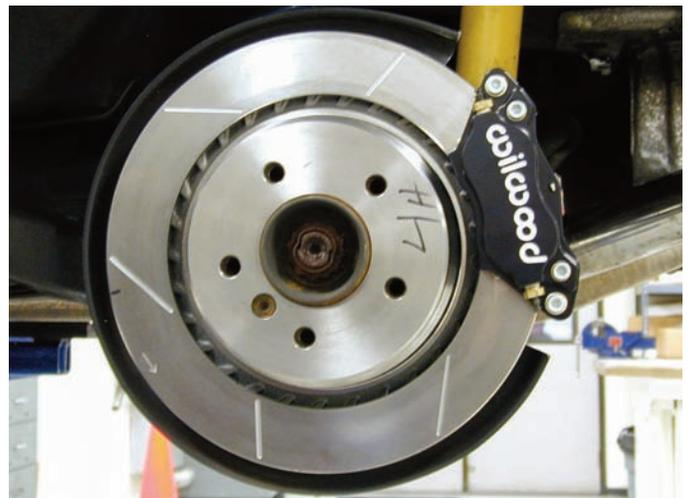
Here is the rear brake assembly finished and ready for action on the street or on the track. The four-piston rear brakes will work perfectly with the larger six-piston front brakes to provide perfect front to rear brake bias. Now the brake bleeding and pad bedding can begin.
