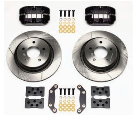
The Wilwood Engineering part number 140-8797 front disc brake kit for the BMW includes the Billet Narrow SL6 Radial Mount calipers, the 13.06-inch slotted rotors, the aluminum hat adapters, the caliper brackets, the BP-10 Smart Pads and all of the hardware required to finish the installation.
