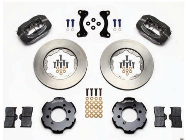
The Miata's brake system was improved with a part number 140-11704 Brake Installation Kit. The kit features forged billet Dynalite four-piston calipers in a black finish. The calipers work together with the 11-inch vented rotors with aluminum hats. The kit includes the caliper brackets, BP-10 brake pads and all of the hardware required to finish the installation.
