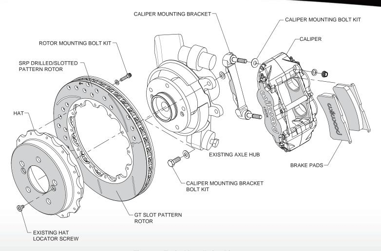
Figure 1. Typical Installation Diagram
