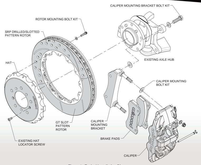
Figure 1. Typical Installation Diagram
