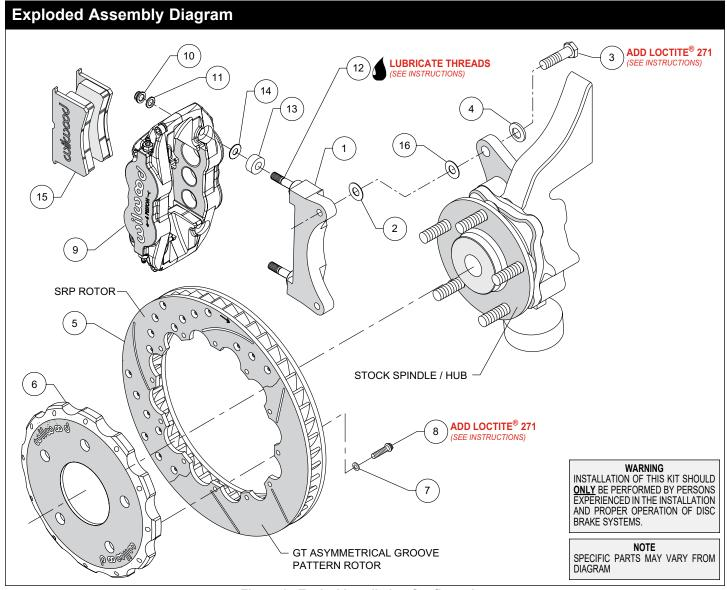
Figure 1. Typical Installation Configuration
