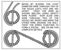
Figure 3. Safety Wire Diagram
