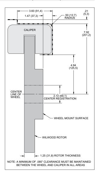
Figure 2. Wheel Clearance Diagram
