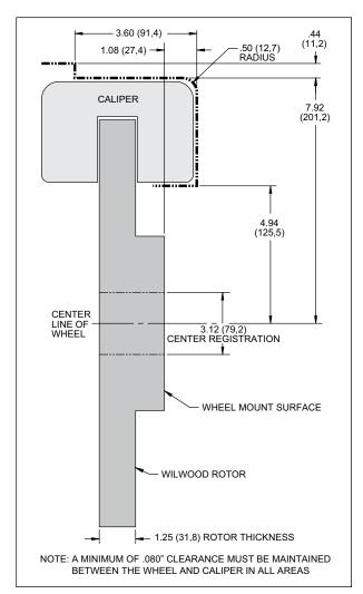
Figure 2. Wheel Clearance Diagram
