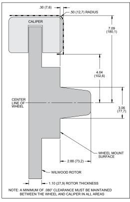
Figure 2. Wheel Clearance Diagram
