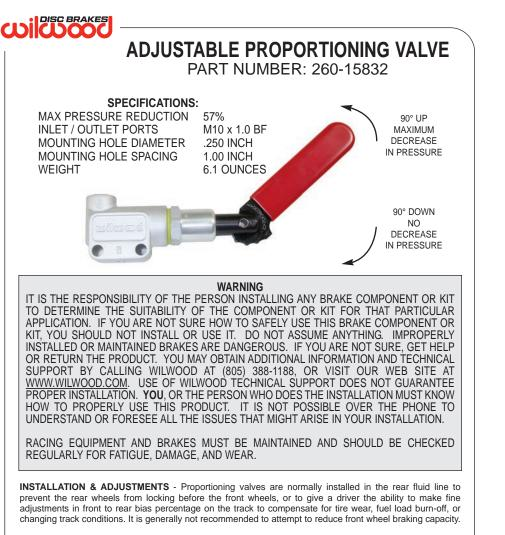
Use only the two .25" body holes to secure the valve to a mount. Do not attempt to remove the adjuster lever or valve body end cap to facilitate thru-panel mounting.
