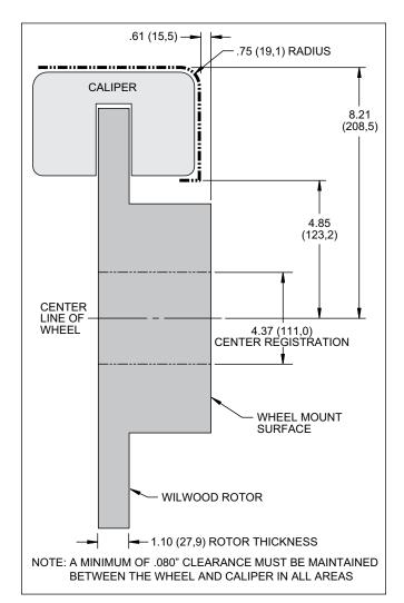
Figure 2. Wheel Clearance Diagram
