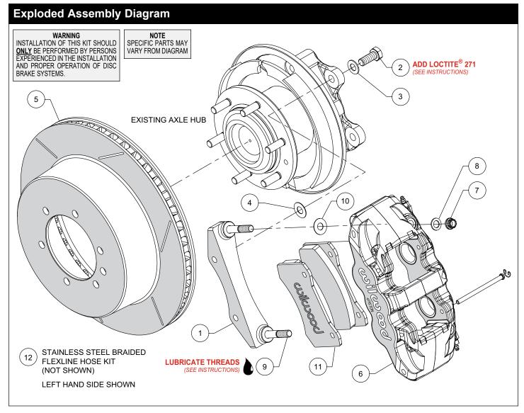
Figure 1. Typical Installation Configuration
