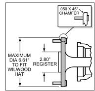
Figure 3. Axle Flange Maximum Dimension
