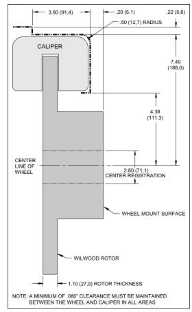
Figure 2. Wheel Clearance Diagram
