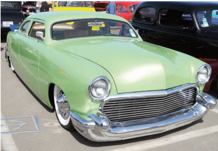
Marty Wells brought out his awesome pearl mint green '51 Ford custom to the show from Yorba Linda, California. The car features a chopped top, it was nosed and decked, the door handles were shaved and it has a custom grille featuring a bumper from a '57 Chevy.
