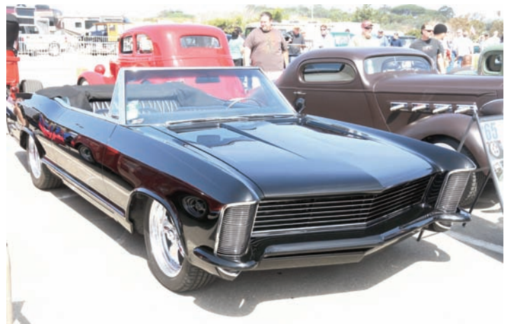
You are looking at one of none. Frank Dobbs from Temecula, California thought a '65 Buick Riviera would be cool so he made his own and it looks like the factory did it. The car also sits nice and low, runs large diameter wheels with low profile tires and a dual-quad 401ci engine provides the power.
