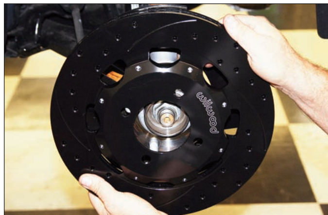
Sequence 12: Install the hat/rotor assembly over the hub assembly. NOTE: The hat/rotor must fit flush against the axle hub flange or excessive rotor run out may result.
