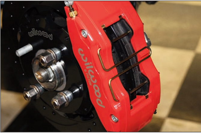
Sequence 19: Secure brake pads in place with the pad clip retainer.
