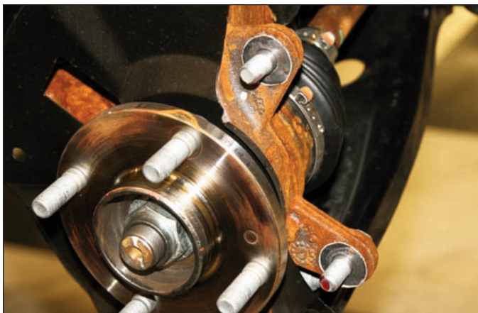
Sequence 7: Slide the caliper bracket mounting bolts with washer thru OEM caliper mounting ears from the inboard side.
