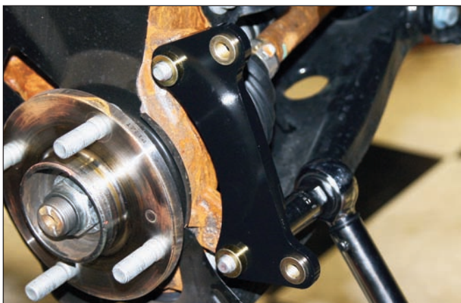
Sequence 8: Attach the Wilwood caliper mounting bracket to the OEM mounting ears on the outboard side. Temporarily tighten the mounting bolts. NOTE: The bracket must fit squarely against the mounting ears. Inspect for interference from casting irregularities, burrs, etc. Grind as necessary. Remove the bolts one at a time and coat with red Loctite ® 271, torque to 60 ft-lbs.
