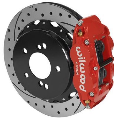
Rear brake kit, P/N 140-14752-DR Download a high resolution photo, click here
