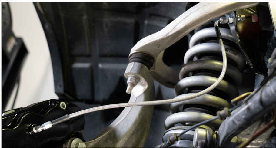
Photo 9 Flexline routing (TRX model not shown)
