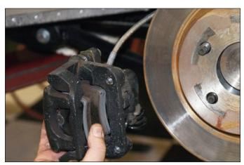
**Sequence 5**: Disconnect the parking brake cable. Lift off the caliper and keep the OEM brake line hose in the vertical position to avoid spilling brake fluid that remains in the hose.
