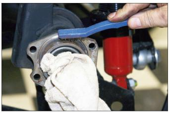
**Sequence 10**: Clean the axle hub with a wire brush and remove any nicks, burrs, or grease that may interfere with the installation of the new flat caliper mounting bracket.
