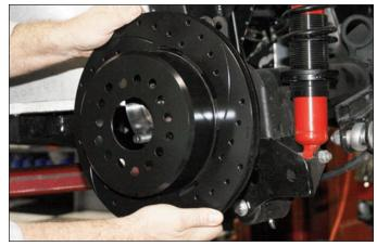
**Sequence 15**: Install the hat/rotor over the axle hub assembly. **NOTE**: The hat/rotor must fit flush against the axle hub flange or excessive rotor run out may result.
