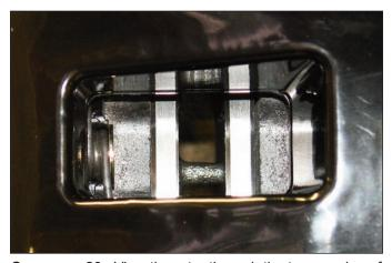
**Sequence 20**: View the rotor through the top opening of the caliper. The rotor should be centered in the caliper. If not, adjust by adding or substracting shims between the caliper mounting bracket and the flat bracket. Once the caliper alignment is correct, remove the bracket bolts one at a time and apply red *Loctite*® 271 to the threads and torque to 22 ft-lb.
