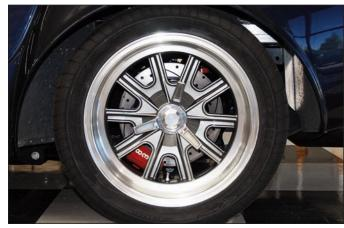
**Sequence 23**: Install the wheel and torque the lug nuts to manufacturer's specification. Rotate the wheel and check for any interference. Reinstall the replica knock-off's. Bed in the brake pads and rotor in a safe location before general use driving.
