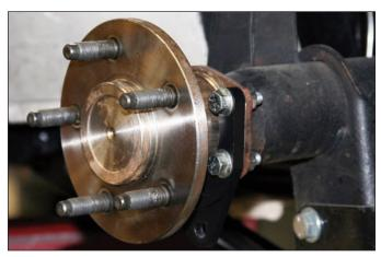
**Sequence 12**: Slide the axle into the rear end housing and connect at the differential per OEM specifications. Refill the differential with OEM specified lubricant.
