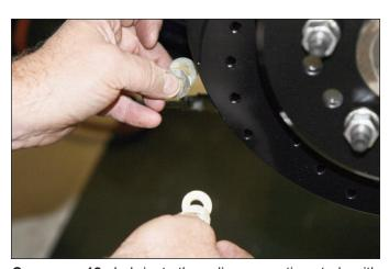
**Sequence 18**: Lubricate the caliper mounting studs with lightweight oil. Initially place two shim washers on each stud between the caliper mounting bracket and caliper.
