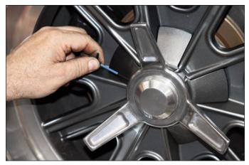
**Sequence 1**: Raise the rear wheels off the ground and support the rear suspension according to the vehicle's manufacturer's instructions. Loosen the set screw behind the replica knock-off and lift off knock-off.
