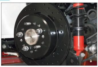
**Sequence 16**: Secure the hat/rotor with three lug nuts (finger tight) to keep the hat/rotor in place while continuing with the installation.
