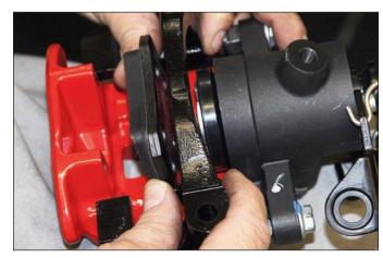
**Sequence 17**: Slide the brake pads up into the caliper from the bottom with the friction material facing the rotor until the "V" spring clip snaps into place against the anvil.
