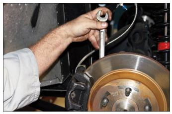
**Sequence 4**: Using a wrench, break loose the caliper mounting bolts from the back side of the rotor.
