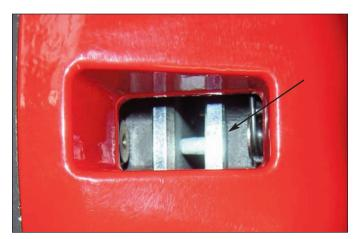
**Sequence 21**: Check that the top of the brake pad is flush with the outside diameter of the rotor (arrow). If not, adjust by adding or substracting shims between the bracket and the caliper. After bleeding (sequence 22), reinstall caliper and torque caliper nuts to 35 ft-lb.
