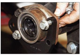
**Sequence 11**: Install the flat housing mount caliper bracket onto the axle hub using bolts, washers, and nuts with the "U" opening in the up position and the mounting ears facing toward the front of the vehicle. **NOTE:** The bracket must fit squarely against the housing flange. Inspect for interference from casting irregularities, burrs, etc. Grind as necessary.
