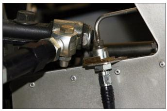
**Sequence 21**: Connect one end of the flexline to the previously installed caliper fitting. Route line along the same path as the OEM hose and connect the other end of the flexline to the fitting at the brake hard line. Secure line as necessary to prevent contact with moving suspension, brake, or wheel components. Bleed the system referring to the additional information in the data sheet as necessary for proper bleeding instructions.
