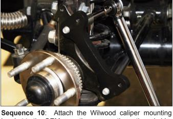
**Sequence 10**: Attach the Wilwood caliper mounting bracket to the OEM mounting ears on the outboard side. Temporarily tighten the mounting bolts. *NOTE:* The bracket must fit squarely against the mounting ears. Inspect for interference from casting irregularities, burrs, etc. Grind as necessary. Remove the bolts one at a time and coat with red *Loctite*® 271, torque to 65 ft-lbs.
