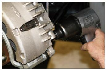
**Sequence 4**: Using an impact driver or breaker bar and socket, break loose the caliper mounting bolts from the back side of the rotor.
