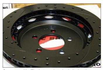
**Sequence 11**: The hat needs to be bolted to the rotor. Orient the rotor over the hat in the configuration shown above.
