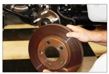
**Sequence 6**: Slide off the rotor from the hub. If it is stuck, it may be necessary to hit it a few times with a rubber mallet to break loose.
