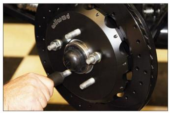
**Sequence 14**: Secure the hat/rotor with three lug nuts (finger tight) to keep the hat/rotor assembly in place while continuing with the installation.
