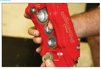
**Sequence 16**: Initially place three shim washers on each bolt between caliper mounting tab and the mounting ears on the bracket.
