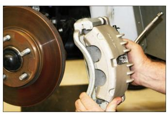
**Sequence 5**: Lift off the caliper and keep the OEM brake line hose in the vertical position to avoid spilling brake fluid that remains in the hose.
