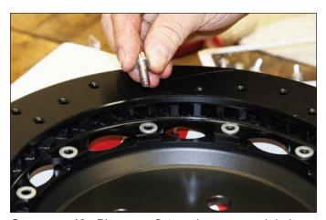
**Sequence 12**: Place one flat washer over each hole on the rotor mounting tabs. Coat the mounting bolts with red *Loctite*<sup>®</sup> 271 and slide through the washer and thread into the hat. Using an alternating sequence, torque bolts to 155 **in-lbs.**
