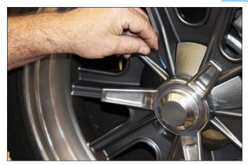
**Sequence 1**: Raise the front wheels off the ground and support the front suspension according to the vehicle's manufacturer's instructions. Loosen the set screw behind the replica knock-off and lift off knock-off.
