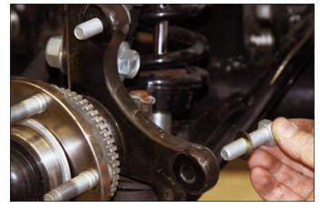
**Sequence 9**: Slide the caliper bracket mounting bolts with washer thru OEM caliper mounting ears from the inboard side.
