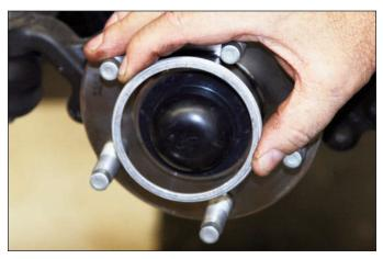
**Sequence 8**: Install the rotor registration adapter over the hub dust cap against the hub face with the larger O.D. facing inward toward the hub face.
