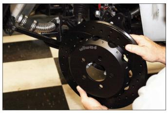
**Sequence 13**: Install the hat/rotor assembly over the hub assembly. **NOTE:** The hat/rotor must fit flush against the axle hub flange or excessive rotor run out may result.
