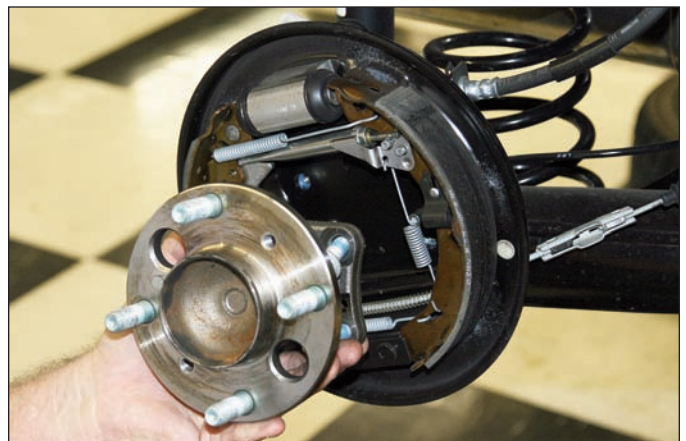
Sequence 5: Lift off the axle hub and set aside.
