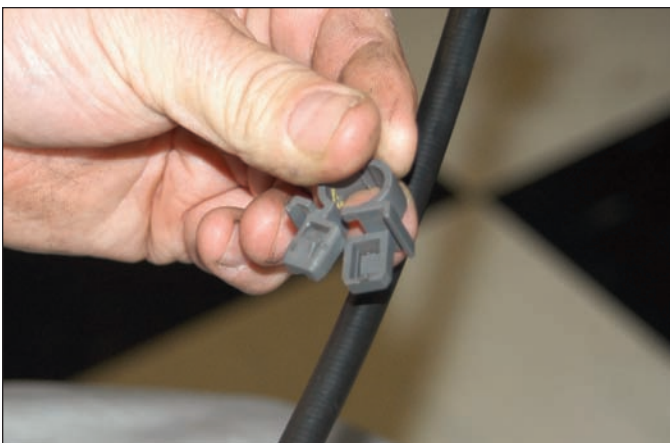
Sequence 1: Install the OEM brackets over the Wilwood cable in the same position that they were removed from the original cables.
