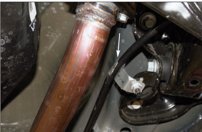
Sequence 5: Secure the cable using the same metal bracket near the exhaust (arrow).
