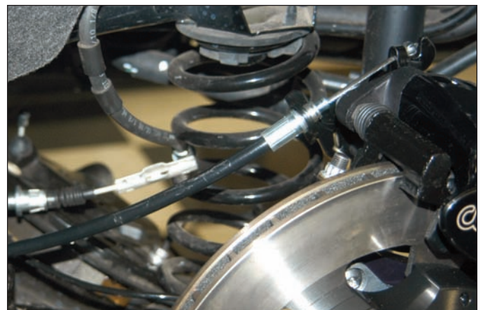
Sequence 2: Attach E-clip end of the Wilwood cable to the parking brake caliper.
