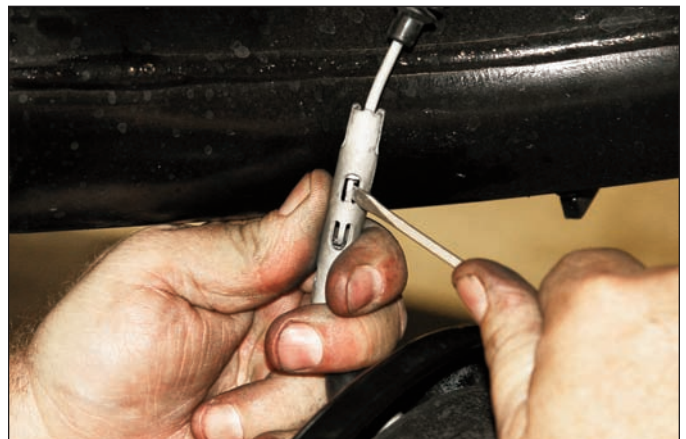
Sequence 6: Disconnect the parking brake cable from behind the drum assembly.
