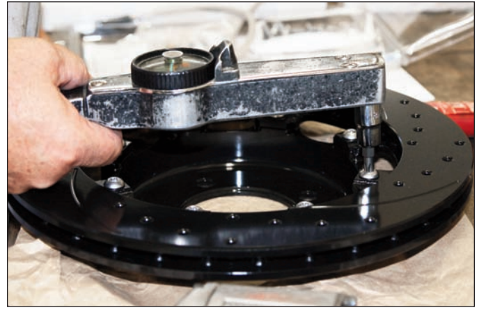
Sequence 16: Using an alternating sequence, torque rotor bolts to 25 ft-lb.
