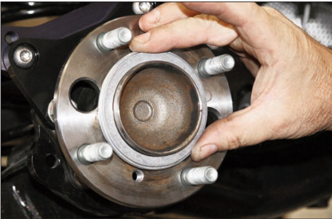
Sequence 14: Install the rotor registration adapter over the axle register against the hub face with the larger O.D. facing inward toward the hub face.
