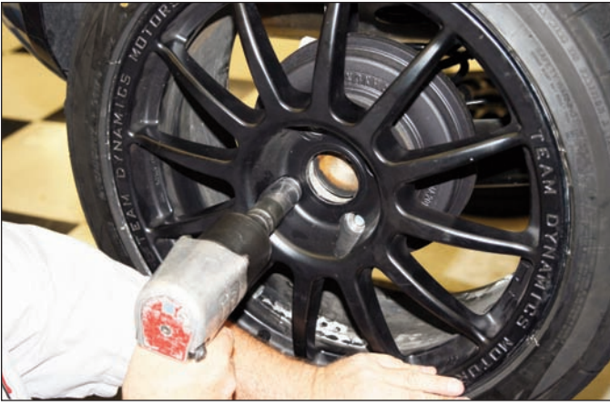
Sequence 1: Raise the rear wheels off the ground and support the rear suspension according to the vehicle manufacturer's instructions. Remove the lug nuts and lift off the wheel.
