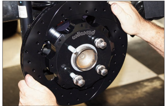
Sequence 17: Install the hat/rotor over the axle hub assembly. NOTE: The hat/rotor must fit flush against the axle hub flange or excessive rotor run out may result. Secure the hat/rotor with three lug nuts (finger tight) to keep the hat/rotor in place while continuing with the installation.
