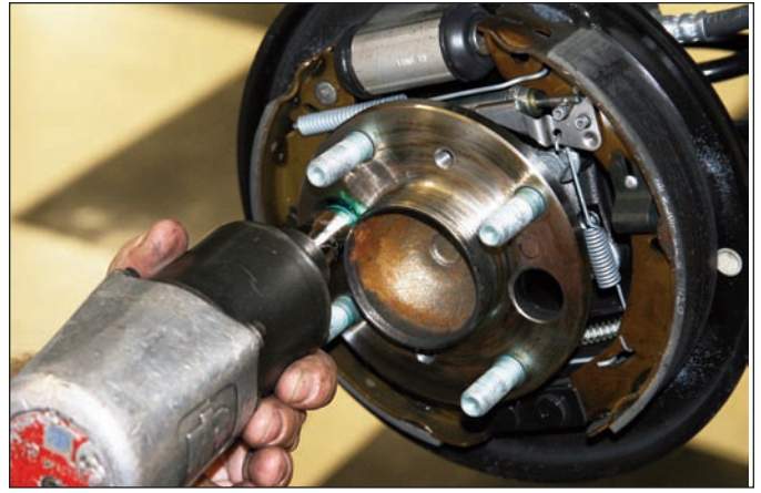
Sequence 4: Using the access holes in the face of the axle hub, remove the nuts holding the axle hub in place.
