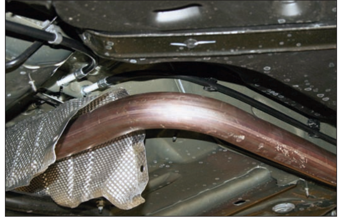
Sequence 8: Final installation of cables to balance bar. Adjust the cable in the bulkhead so it is approximately centered in its adjustment range.
