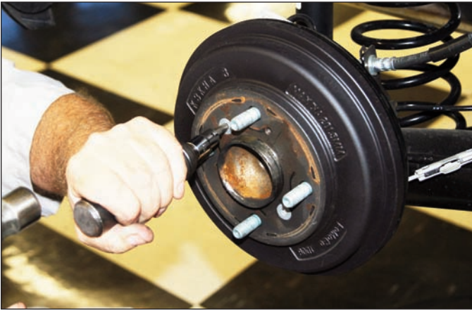
Sequence 2: Break loose the hat locator screw using an impact screwdriver. Then remove the screw.
