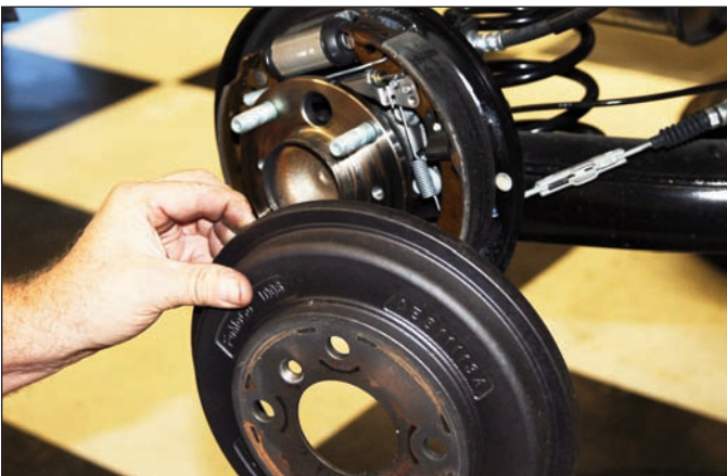
Sequence 3: Slide off the drum from the parking brake assembly.
