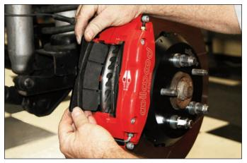
**Sequence 18**: Having already removed the caliper center bridge pad retainer bolt, nut, and tube from the caliper, insert the brake pads into the caliper with the friction material facing the rotor.
