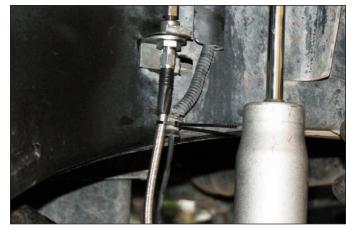
**Sequence 22**: Connect the other end of the flexline to the fitting at the brake hard line. Secure line as necessary to prevent contact with moving suspension, brake, or wheel components. Bleed the system referring to the additional information in the data sheet as necessary for proper bleeding instructions.
