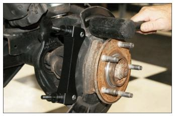
**Sequence 10**: The dust shield needs to be bent backwards slightly for the Wilwood hat/rotor assembly to fit properly. Test fit hat/rotor and bend as necessary to allow a minimum of .12" clearance.
