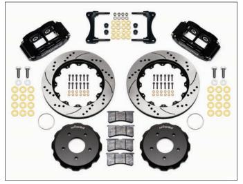
Wilwood part number 140-12440 comes complete with Superlite 4R calipers, caliper mounting brackets, GT rotors, aluminum hats, BP-10 brake pads and all necessary hardware for an easy bolt-on installation.
