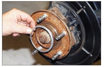
**Sequence 7**: Install the rotor registration adapter over the hub against the hub face with the larger O.D. facing inward toward the hub face.
