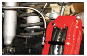
**Sequence 21**: Connect one end of the Wilwood flexline hose kit, P/N 220-11237 to the fitting that was previously installed into the caliper. Route the line along the same path as the old rubber OEM line.
