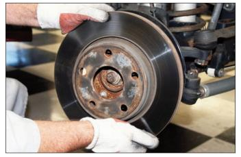
**Sequence 4**: Slide off the rotor from the hub. If it is stuck, it may be necessary to hit it a few times with a rubber mallet to break loose.
