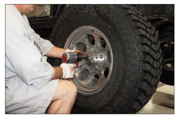
**Sequence 1**: Raise the front wheels off the ground and support the front suspension according to the vehicle's manufacturer's instructions. Remove the lug nuts, then slide off the wheel.
