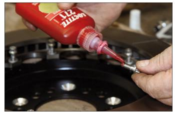
**Sequence 5**: Place one flat washer over each hole on the rotor mounting tabs. Apply red *Loctite*<sup>®</sup> 271 to the mounting bolts and slide through the washer and thread into the hat.
