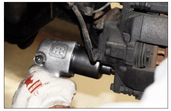
**Sequence 2**: Using a impact gun, or breaker bar and socket, break loose the caliper mounting bolts from the back side.
