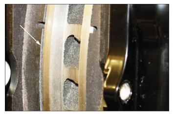
**Sequence 19**: Check that the top of the brake pad is flush with the outside diameter of the rotor (arrow). If not, adjust by adding or substracting shims between the bracket and the caliper.
