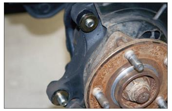
**Sequence 8**: Slide two caliper mounting bracket bolts through the OEM caliper mounting ears from the inboard side and initially install two shim washers on each bolt.
