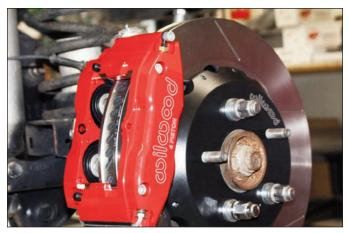
**Sequence 16**: Mount the caliper onto the bracket with the bleed screws in the up position.
