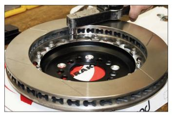
**Sequence 6**: Using an alternating sequence, torque rotor bolts to 155 **in-lbs**.
