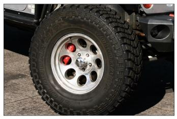
**Sequence 23**: Install the wheel and torque the lug nuts to manufacturer's specification. Ensure the wheel rotates freely without any interferrence. Bed in the brake pads and rotor in a safe location before general use driving.
