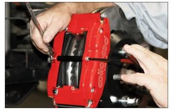
**Sequence 20**: After the pad height is set, install the center bridge pad retainer tub, bolt, and lock nut using an Allen wrench and open-end wrench. The lock nut should be snug without play in the bolt or tube. Be cautious not to over tighten. Then finalize the caliper mounting by torquing the caliper mounting lock nuts to 30 ft-lb.
