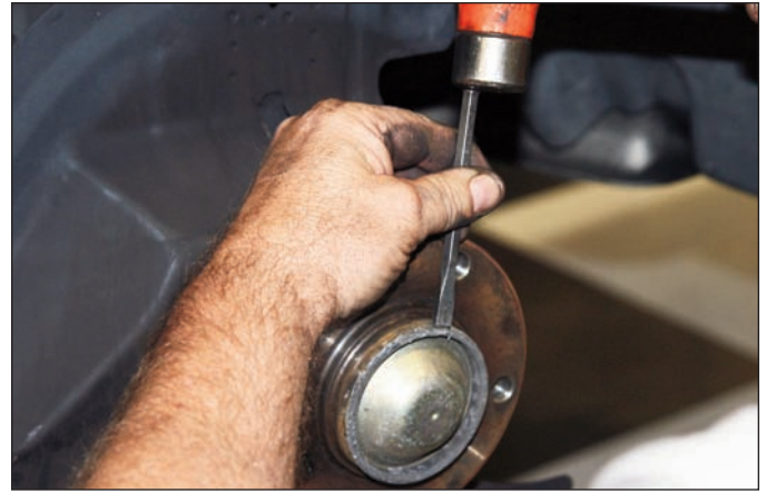
Sequence 10: Pry off the dust cap from the face of the hub using a chisel or screwdriver and a hammer.
