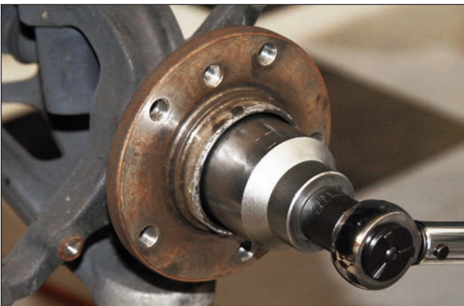
Sequence 15: Install a new OE spindle nut and torque per vehicle manufacturer's instructions.
