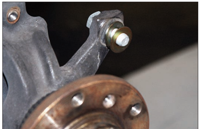
Sequence 18: Slide caliper bracket mounting bolts thru OEM caliper mounting ears from the inboard side. Initially install two shim washers on each bolt between mounting ear and bracket.
