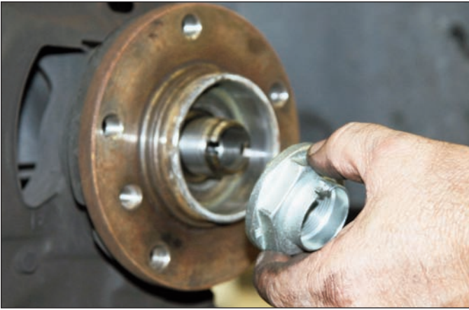
Sequence 13: After the spindle nut is removed, slide off the hub assembly and save for reinstallation later.
