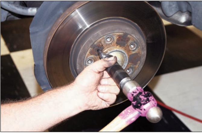
Sequence 7: Break loose the hat locator screw using an impact screwdriver. Then remove the screw.
