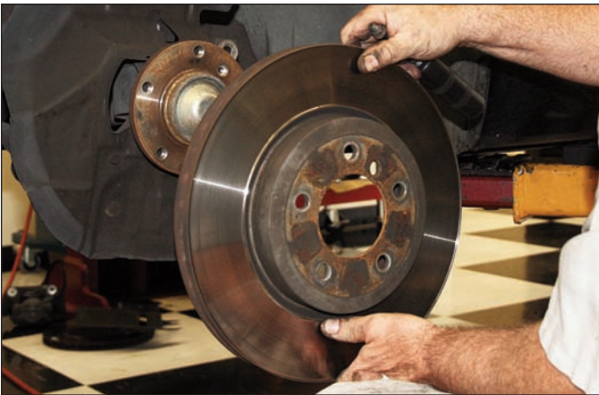
Sequence 8: Slide off the rotor from the hub. If it is stuck, it may be necessary to hit it a few times with a rubber mallet to break loose.
