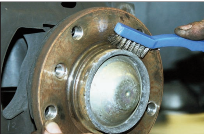
Sequence 9: Clean the hub assembly with a wire brush and remove any nicks, burrs, or grease that may interfere with installation of the new brake components.
