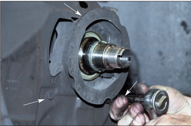
Sequence 14: Remove the three bolts (arrows) that hold the dust shield in place. Remove the dust shield and discard, it will not be utilized in the installation of the Wilwood brake kit.
