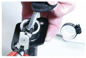
The rubber boot was disconnected from the back of the master cylinder far enough to access the snap ring that holds the piston inside of the bore.
