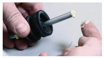
The end of the push rod that rests against the piston assembly was coated with white grease.
