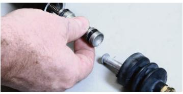
Even with pressure from the spring, the piston assembly will have to be pulled out of the master cylinder.
