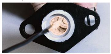
Using a small light, the bore was inspected for scratches and other imperfections that would prevent the unit from working properly. In this case the bore was in good condition and was perfect for a rebuild. If you do find a major problem it would be a good idea to purchase a new unit.
