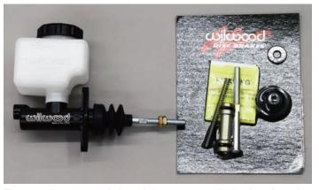
The small and very lightweight master cylinder is a favorite with racecar builders. The rebuild kit makes rebuilding fast and easy, because the kit comes complete with a new spring, a piston assembly that's ready to install, a push rod and a new rubber boot.
