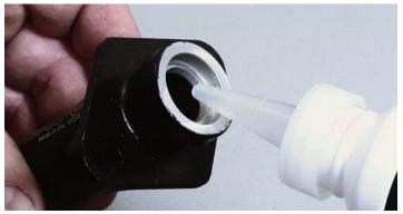
A few drops of Wilwood lubricant was placed inside of the piston bore and then it was distributed evenly inside of the bore. This can be done with finger power.
