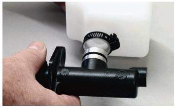
The hose clamp connection was loosened with a screwdriver and then the plastic reservoir was carefully removed from the master cylinder. Notice the O-ring seal that keeps this connection leak free.
