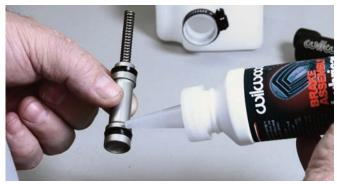
The rubber piston cup seals were coated with lubricant to make it easier to install the piston inside of the master cylinder bore.
