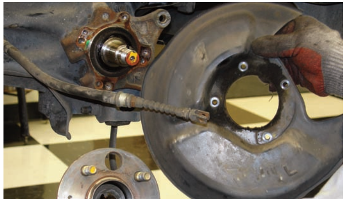
After the hub flange was removed, the dust shield could be removed from the assembly. It will no longer be used for the new brake application. After the dust shield was removed, the hub flange was reattached.
