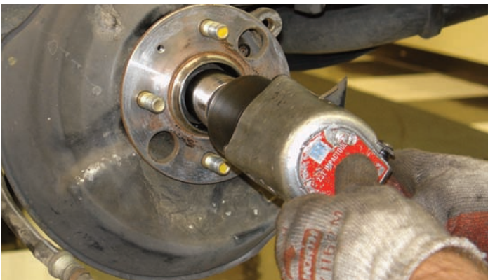
In order to remove the dust shield the hub flange has to be removed. Here the large nut that fastens it was removed with an impact gun.
