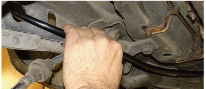
Using the original clips the new Wilwood part number 130-10966 parking brake cables were installed. The new Wilwood part number 120-10840 braided steel lines were also connected to the caliper.
