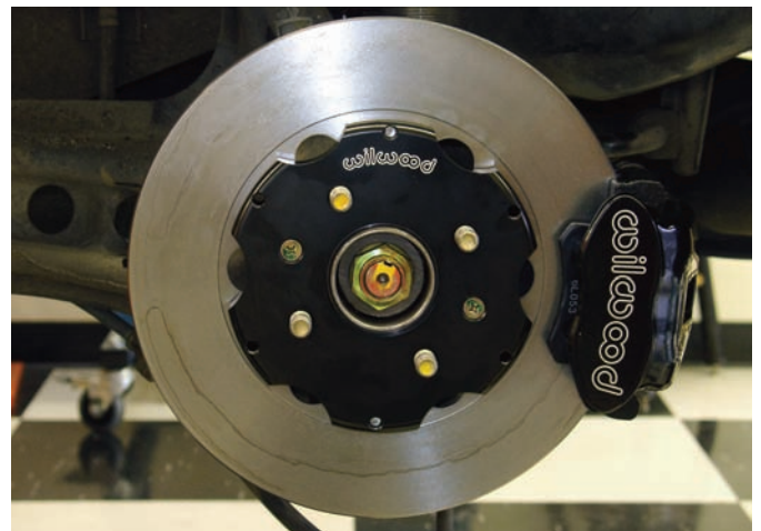
Here is the finished rear brake assembly that is hooked up and ready for brake bleeding and bedding. This rear brake assembly is larger and stronger than the original unit.
