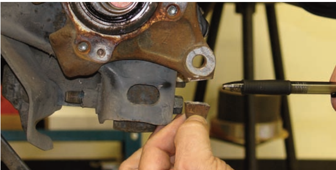
Here is the section that was removed. It is important to only cut off the lower section and not to cut too close to the ear hole because that will weaken the bracket. If you have a grinder you can flatten and radius the part.
