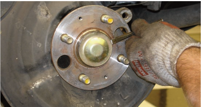
Using a screwdriver or chisel the outer edge of the dust cap was tapped to remove it from the assembly.
