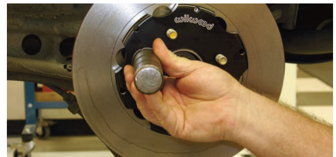
Here is the rotor after the adapter was installed. It was attached to the hub flange using the two original screws that were removed previously. The screws can be tightened using the impact screwdriver.
