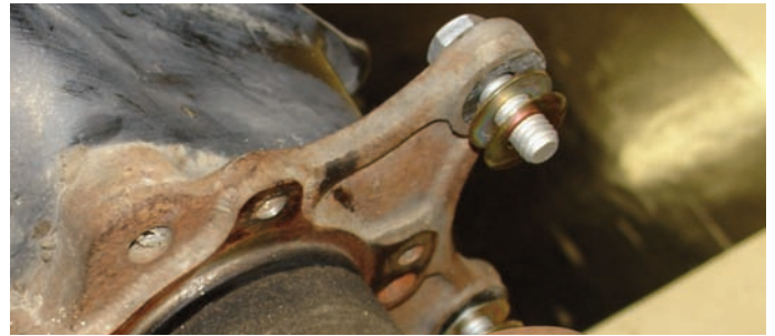
The caliper bracket mounting bolts were placed through the mounting ears and they were loaded with two washers, one 0.016-inch thick and the other 0.035-inch thick. A 0.057-inch thick washer was used under the bolt head.
