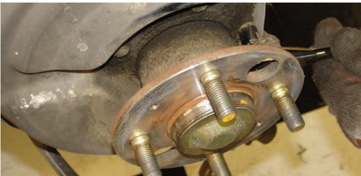
The small bolts that secure the dust shield to the hub assembly were disconnected using a small socket wrench. Some of the small bolts can be accessed through the hole in the flange.
