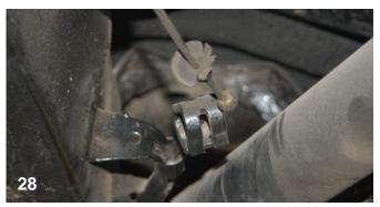
Here is the rear cable after it was disconnected from the main parking brake cable.
