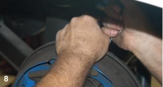
Before the backing plate can be removed from the axle, the brake line has to be disconnected from the wheel cylinder.
