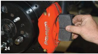
The BP-10 Smart Pads were installed in the calipers as seen here. They drop in from the top, which makes brake pad changes easy.
