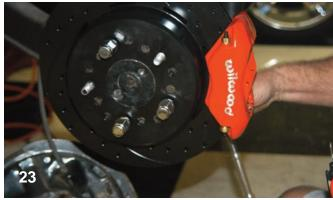
After the caliper mounting bolts were connected finger tight, they were tightened with a socket wrench. After the bolts were tight, the caliper was centered over the rotor.
