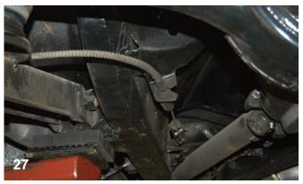
The original emergency brake cable will no longer be used. The cable has to be released and the cable has to be removed from the frame bracket.
