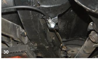
Using a Wilwood universal brake cable kit, a new brake cable mechanism was installed.
