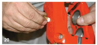
The inlet fitting threads were covered with PTFE Thread Tape and then the fitting was screwed into the caliper.
