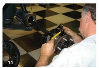
The parking brake assembly was installed on the axle and the bearing retainer holes were lined up with the parking brake mechanism as the unit was slid into place.
