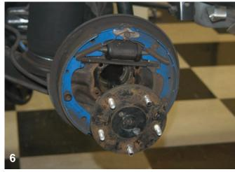
After the four nuts were disconnected, the axle was removed from the differential case. This might require an axle-puller.
