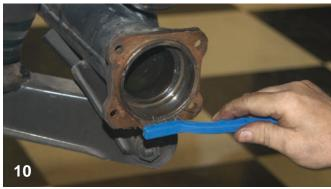
After the backing plate was removed, the axle flange was cleaned with a wire brush. The grease seal in the axle was in good condition so it was retained for this brake installation.
