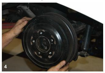
The brake drum was moved side-to-side to release it from the centering ring. After it was loose, it was removed from the car.
