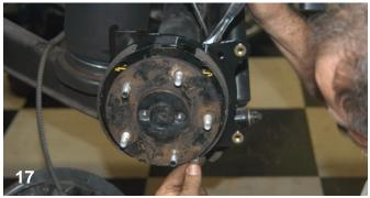
All four bolts were tightened with an open-end wrench on the outside and a socket wrench on the backside. The connection should be very tight, so double-check the connection.
