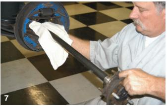
Here Tony is removing the axle from the car. He wipes the excess axle grease off of the axle as it's being removed.
