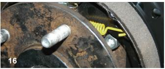
Peeking though the opening, you can see the nut on the bolt. Before the nut was installed, a small flat washer was placed on the bolt. This is a tough area to reach, so you will have to be tricky to get the nut connected to the bolt. Tony used a magnet tool to get the parts started.
