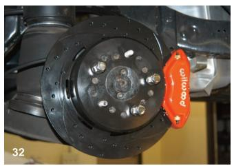
Here is the finished brake assembly ready for action. The Dynapro caliper will work perfectly with the front brake and will provide a good front to rear brake bias. The black rotor face will turn to bare silver metal after a few brake applications are made.
