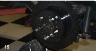
The lug nuts were installed to hold the rotor firmly against the axle flange, so the rotor to caliper centering can be checked.
