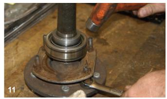
The bolts in the bearing retainer were removed because new bolts will be used for this installation.
