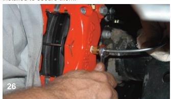
The original rear axle brake line was connected to the fitting in the caliper. Only a small amount of bending was required.
