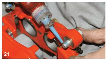
It was determined that only one shim washer was required to center the caliper and rotor. Here the attachment bolt was being coated with Loctite prior to installing the caliper.
