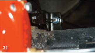
The other end of the universal brake cable hooks to the bracket on the parking brake mechanism and to the arm that activates the system.
