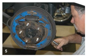
The four nuts and bolts that connect the bearing retainer and backing plate to the axle flange were disconnected. Here the bolts are being loosened with a breaker bar.
