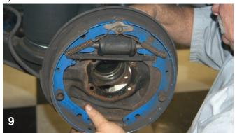
After the connection to the wheel cylinder was disconnected, the backing plate was removed from the axle.
