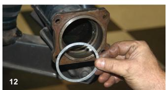
The kit comes with this bearing spacer that fits snugly inside of the axle tube.
