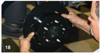
The black E-Coated rotor was placed on the studs and was slid back until the opening in the rotor was firmly against the axle flange centering ring. Notice the additional holes that are used to line up with other lug bolt configurations.
