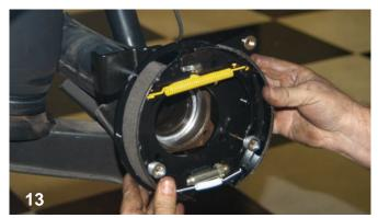
The parking brake mechanism was placed against the axle opening to make sure the boltholes line up properly.
