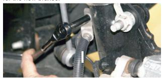
The original rubber brake lines were removed in preparation of installing the Wilwood Flexlines. The bracket by the strut was disconnected and it will be modified to work with the Wilwood lines.
