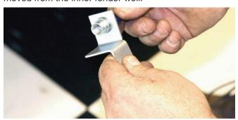
Similar to the way the front bracket was modified, this one was opened up so that it would accept the fitting shown here. After that was finished the bracket was bolted back into the original location with one side of the fitting connected to the steel line.
