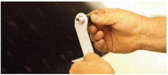
The hole in the bracket was opened up so that this fitting could be installed. It will be held in place with a brake line clip.
