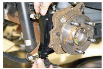
After the intermediate caliper bracket was installed, the main caliper bracket was bolted to the intermediate bracket.
