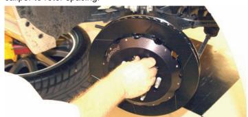
After the Wilwood caliper bracket was secured, the E-coated rotor was attached to the hub and spindle assembly.
