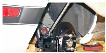
The correct amount of shims and washers were installed to get the caliper centered over the rotor. Here the caliper mounting nuts were coated with Loctite 271 and were tightened to 30 ft-lbs.
