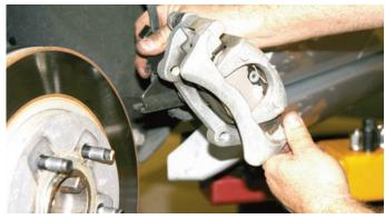
After the caliper bolts were removed, the heavy cast iron caliper was lifted up and was removed away from the car.
