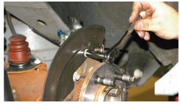
Using a small ratchet wrench and the appropriate size socket, the dust shield bolts were removed.
