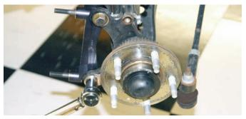
The rotor and caliper were removed so that the caliper bracket bolts could be accessed. Here the bolts were coated with Loctite 271 and were tightened with a torque wrench to 47 ft-lbs.
