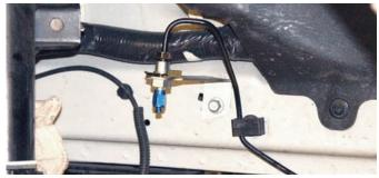
Here is the bracket with the steel line and fitting installed, and ready for the braided steel Wilwood Flex line. Here you can see the brake line clip that holds the fitting in place.
