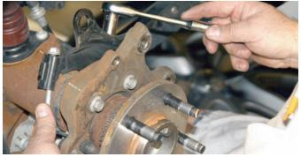
After all of the bolts were disconnected, the dust shield was removed and it will not be reused.
