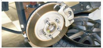
The wheels were reinstalled and the front of the car was lowered. After the front of the car was on the ground, the rear of the car was raised and jack stands were installed under the differential. The wheels and tires were removed to reveal the rear brakes.
