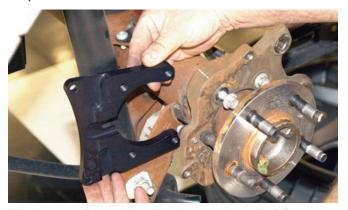
The intermediate caliper bracket was installed first as seen here.
