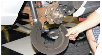
After all of the bolts were disconnected, the dust shield was removed and it will not be reused.
