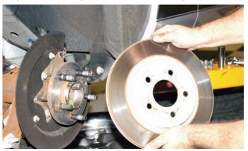
The rotor was removed from the rear axle flange as seen here. Some light tapping with a rubber mallet will help loosen the connection.
