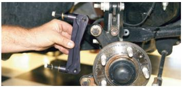
The Wilwood caliper bracket was bolted to the original caliper mounting holes in preparation for getting the proper caliper to rotor spacing.
