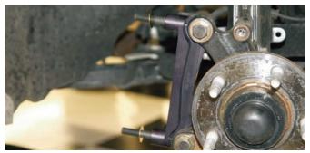
The caliper bracket studs were coated with oil and then they were loaded with the appropriate washers and spacers before the caliper was installed.
