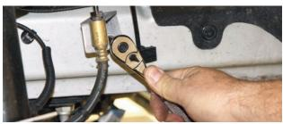
The original frame bracket, where the steel line mates to the rubber line, was disconnected so that it can be modified to work with the Wilwood braided steel Flexline.
