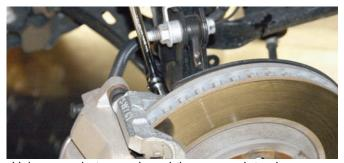
Using a socket wrench and the appropriate size socket, the two bolts and washers that fasten the caliper to the bracket were disconnected. This is a heavy cast iron caliper, so the Wilwood brake kit with aluminum calipers will lower the weight of the car.
