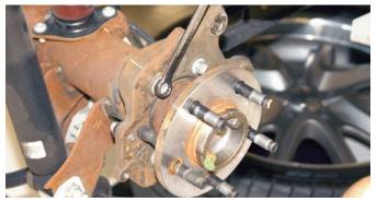
This original caliper bracket bolt was removed because it will be used to connect the Wilwood intermediate caliper bracket.
