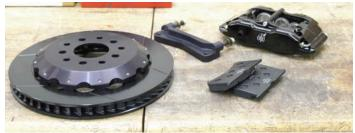
The rotor and the hat were bolted together using the ¼-20 bolts and corresponding washers in the kit. The bolts were tightened to 85 in-lbs and then they were safety wired using standard 0.032-inch diameter stainless steel safety wire. The rotor, caliper, caliper brackets and pads were placed on a bench prior to installation for easy access.
