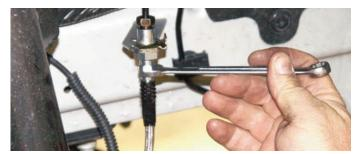
The Wilwood braided steel Flexline was routed between the bracket on the frame and the fitting on the caliper, making sure that it doesn't interfere with any moving parts.
