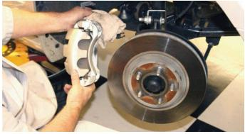
After the bolts were disconnected, the heavy caliper could be lifted off of the bracket assembly.
