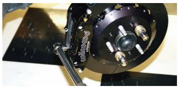
After it was determined that the caliper was positioned correctly, the mounting nuts were tightened to 35 ft-lbs. The wheels and tires were reinstalled and the front of the car was lowered.
