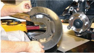
The dust shield was removed from the car and it won't be reused. After the upright is removed it would be a good time to clean any dirt from the "hat locator" and lugs on the hub.
