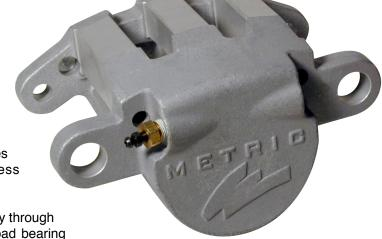
The caliper body is a precision casting using a tight grained, high density aircraft alloy. Stainless steel pistons provide improved fluid protection with high resistance to corrosion and low heat transfer. Each caliper is fully machined, assembled with high temperature seals, and tested in-house by expert Wilwood technicians to assure top quality and peak performance – the kind of quality and performance you expect from Wilwood.
