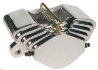
Calipers are fitted with high temperature square piston seals to control piston retraction and stainless steel deep cup pistons reduce heat transfer from the pad to the brake fluid. The caliper accepts 1/8-27 NPT inlet fitting and comes standard with our exclusive re-usable pad retainer clip.
