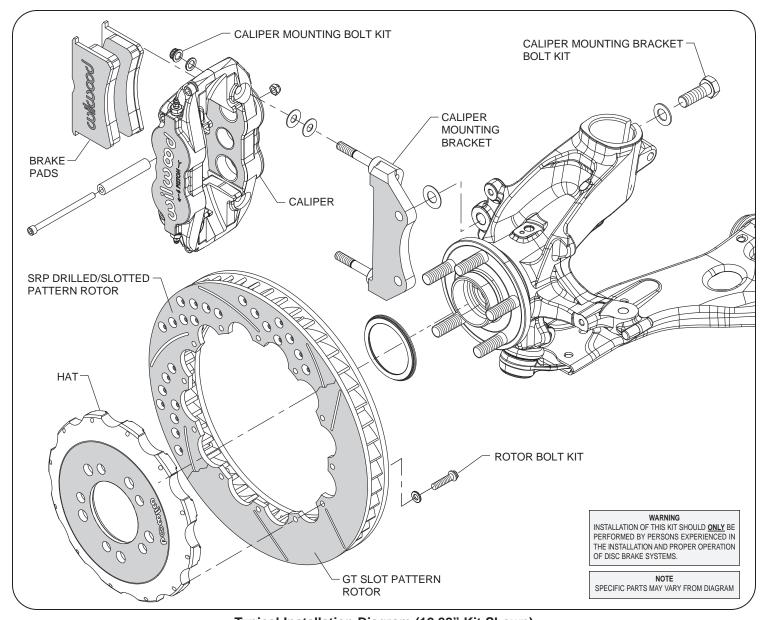
Typical Installation Diagram (12.88" Kit Shown)
